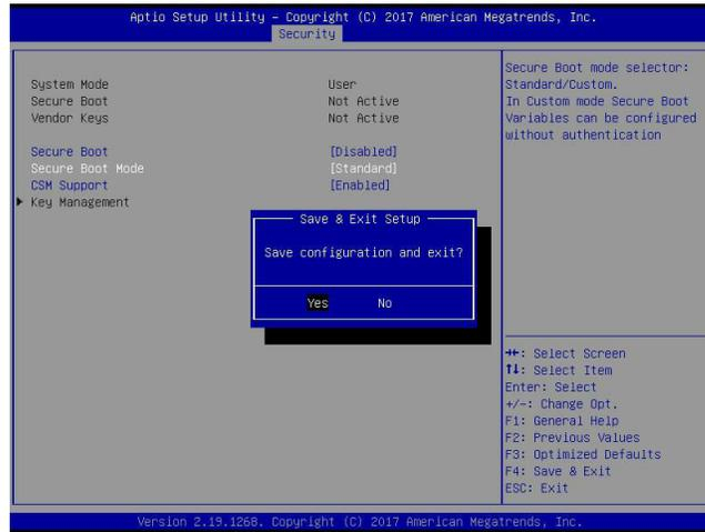
Step 3. Press <Del> during system boot to enter the BIOS Setup utility. Navigate to the Security tab and enter the Secure Boot menu. Set CSM Support to Disabled.
