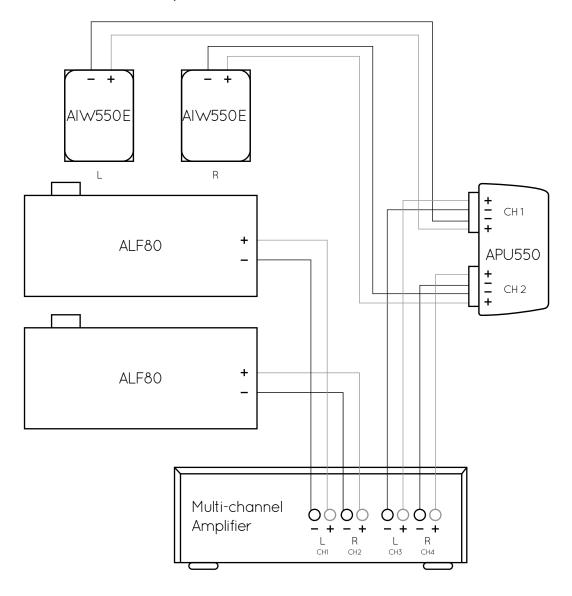
For systems using a pair of AIW550E speakers in rooms larger than 75m<sup>2</sup> two ALF80's will be necessary. In this scenario the amplifier will need four independent channels.
