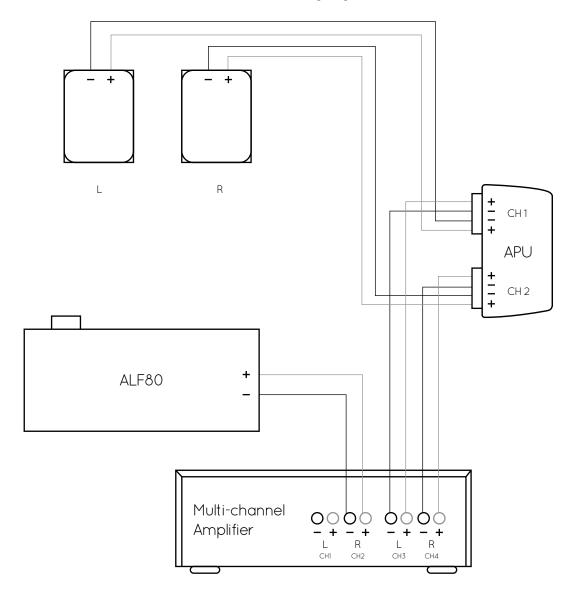
By connecting a single ALF80 to its own amplifier channel, its output (relative to the invisible speaker pair) can be set optimally. In larger rooms care should be taken not to adjust the relative output of a single ALF80 too high. This may result in the unit reaching its mechanical limits well before that of the accompanying invisible speakers. In a larger room (>75m²) a second ALF80 may be required.
