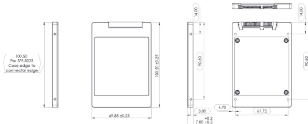
The figure below is enlarged to show detail, but is not the actual size of the form factor. This figure shows 2.5"/7mm cased one-half form factor (for 250GB and 512GB capacities only).
