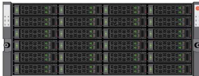
Nimble Storage AF1000 All Flash Array (Base array, 4U; all 24 bays hold Dual Flash Carriers with Small Form Factor SSDs)
