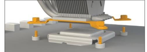
on the rear side of the motherboard into the hexagonal nuts with sleeve (6) attached to the cooler.
