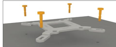
Fasten the backplate on the front side of the motherboard using the C-profile spacers (12) by pressing these onto the notches in the M3x16 screws (9) until they click in.
