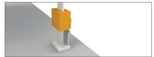
Position the cooler so that it is possible to attach the cooler by screwing together the M3x16 screws (9)
