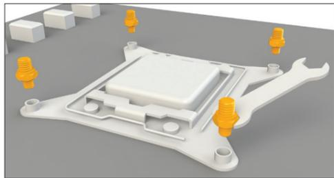
**Installation of the mounting brackets**
