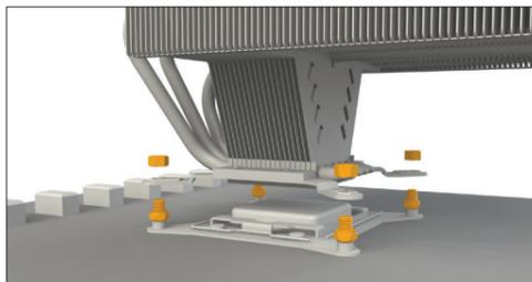
Place the hexagonal nuts (8) over the spacer nuts (7) and progressively tighten these in a crosswise manner until firm using the hexagonal wrench (14).
