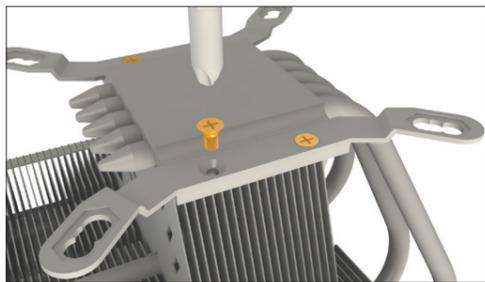
**Mounting the CPU cooler**
