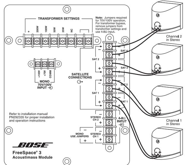
Using 4 satellite speakers with direct connections
