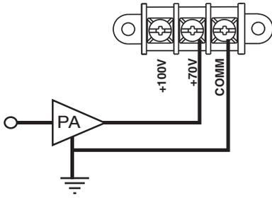
Jumpers in the factory-installed configuration for 200W use.
