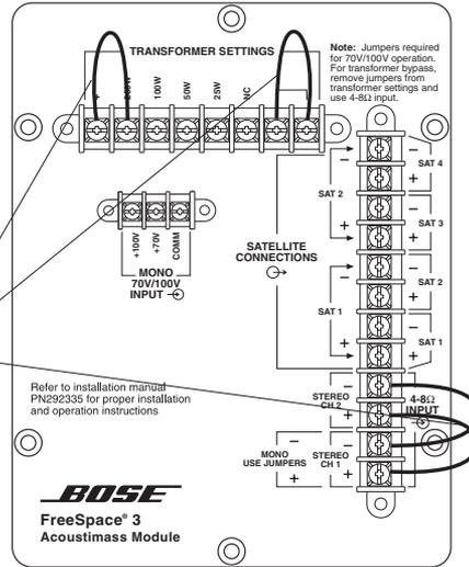
The transformer tap setting from the factory is for 200W use. To set it for lower wattage, remove the end of the '+' jumper wire connected to 200W and reattach it to the appropriate tap (100W, 50W or 25W).
