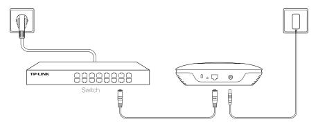
Plug one end of the provided power adapter into the POWER port of the EAP and the other end to a standard
