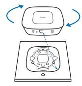
Attach the EAP to the mounting bracket by aligning the arrow mark on the EAP with the arrow mark on the mounting bracket, then rotate the EAP as shown until
