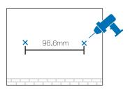
Make two small pencil marks on the wall. Make sure the two marks are level and should be 98.6mm apart. Drill two 6mm holes through the center of your marks.
