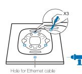
Place the mounting bracket in the center of the ceiling tile. Mark the three positions of the screw holes and a 10mm hole for the Ethemet cable to feed through. Drill three 4mm holes and a 10mm hole for the Ethernet
