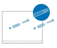
Insert the plastic wall anchors into the 6mm holes and drive the self-tapping screws into the anchors. Do not drive the screws all the way in and leave enough clearance to hang the EAP.
