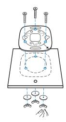
Secure the mounting bracket to the ceiling tile using three M3x30 pan-head screws, washers and wing nuts, as shown on the left.
