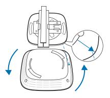
Attach the EAP to the mounting bracket by aligning the arrow mark on the EAP with the arrow mark on the mounting bracket, then rotate the EAP as shown until it locks into place.
