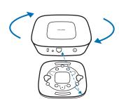
Attach the EAP to the mounting bracket by aligning the arrow mark on the EAP with the arrow mark on the mounting bracket, then rotate the EAP as shown until it locks into place.
