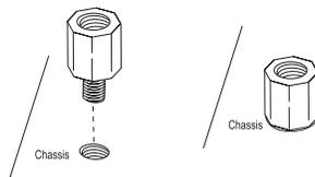
3. Locate the matching mounting holes on the chassis. Align the mounting holes on the motherboard against the mounting holes on the chassis.
