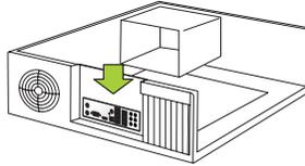
2. Locate the mounting holes on the motherboard. See the previous page for the location.
