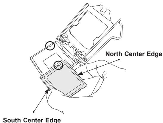
4. Align the CPU key that is the semi-circle cutouts against the socket keys. Once it is aligned, carefully lower the CPU straight down into the socket. (Do not drop the CPU on the socket. Do not move the CPU horizontally or vertically.)
