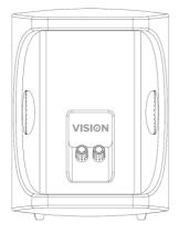
4. TIGHTEN BRACKET SCREWS Set desired angle and lock off side screws.
