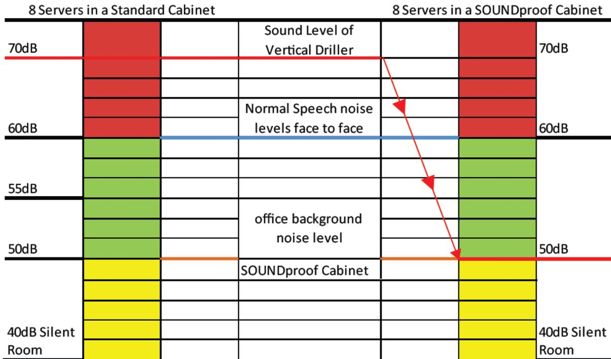
18-21 dB noise level reduction from 1 meter distance to the enclosure
