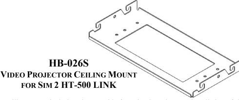
The Chief HB-026S video projector ceiling mount is designed to provide fast, simple and secure installation of the SIM 2 HT-500 LINK, Special roll, pitch, yaw and horizontal adjustments simplify projection positioning for image alignment. The HB-026S mount also has positive registration lock so that the projector may be removed without losing projector mount registration.
