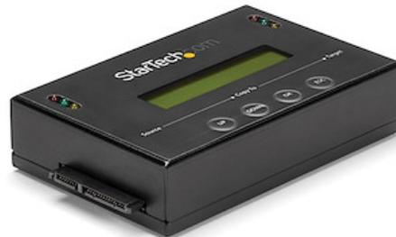
The SATDUP11 standalone hard drive duplicator eraser enables you to copy 1-to-1, or erase up to 2 SATA hard drives simultaneously without a host computer.
