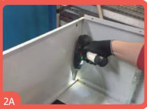
2-Mount the rear panel to the lower frame with two pieces of M5x12 screws each.
