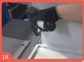
1-Mount the side panels on the lower frame with two pieces of M5x12 screws each.
