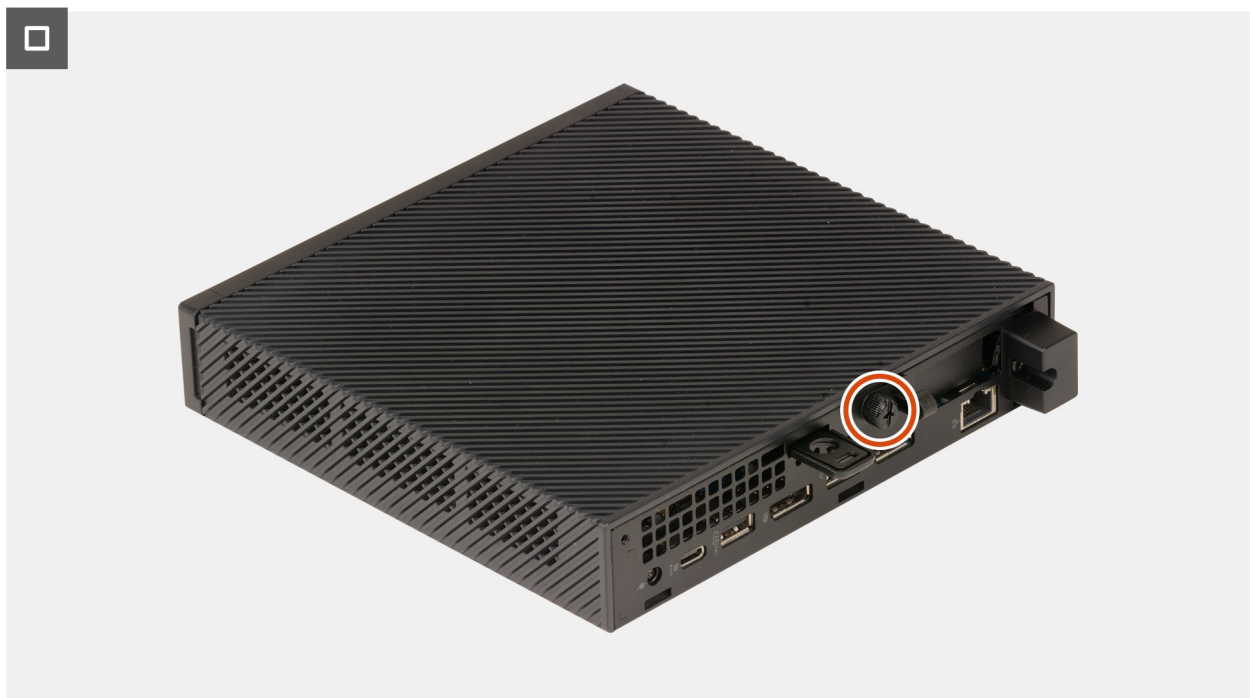
Figure 7. Installing the side cover
