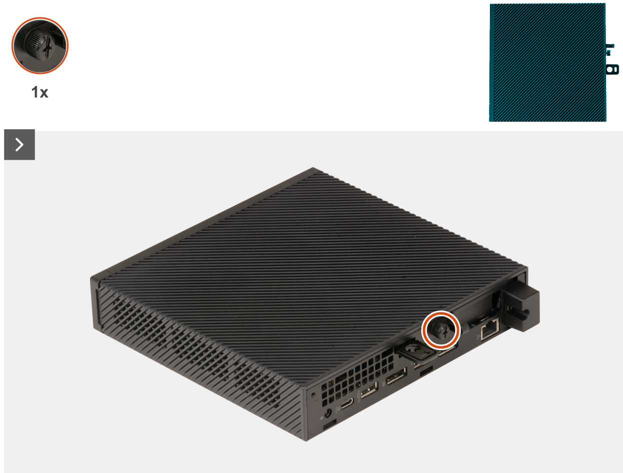
Figure 2. Removing the side cover
