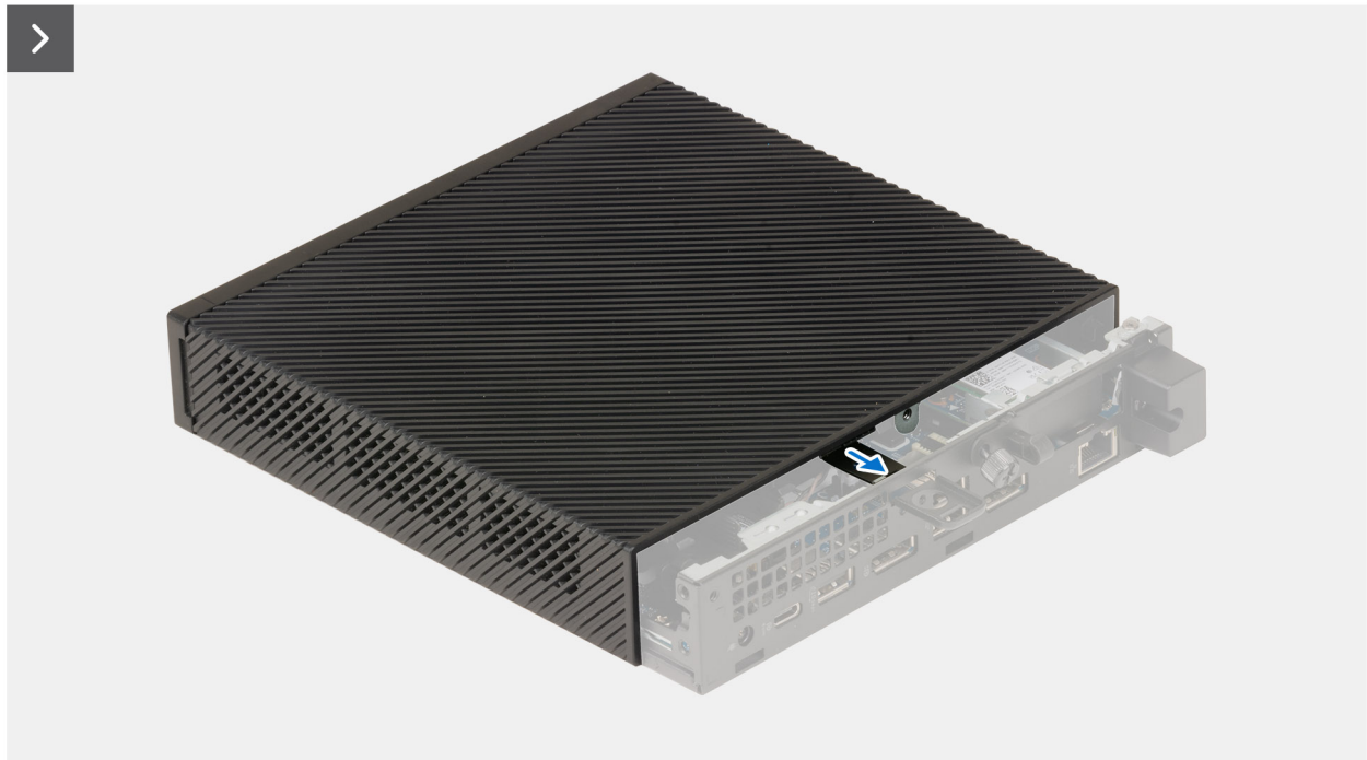
Figure 6. Installing the side cover
