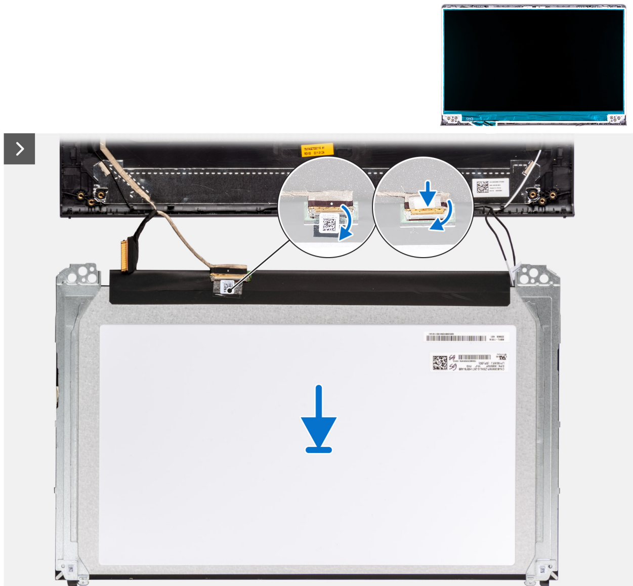
Figure 55. Installing the display panel
