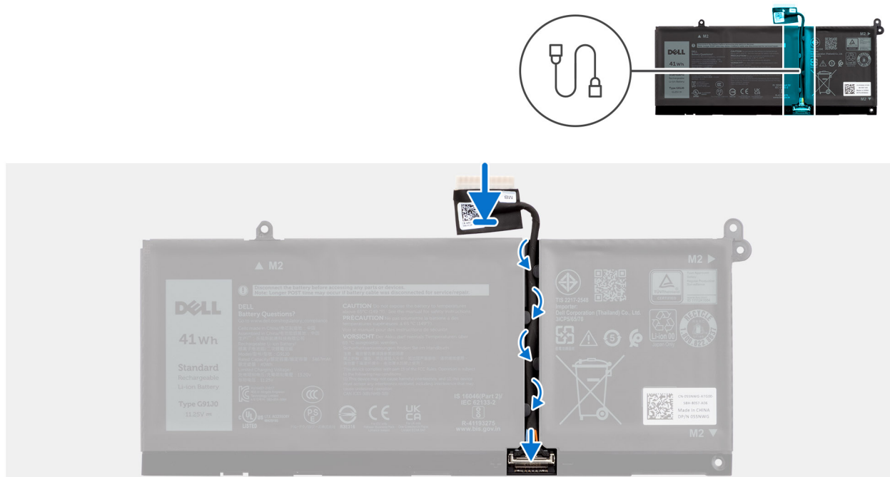
Figure 13. Connecting the battery cable
