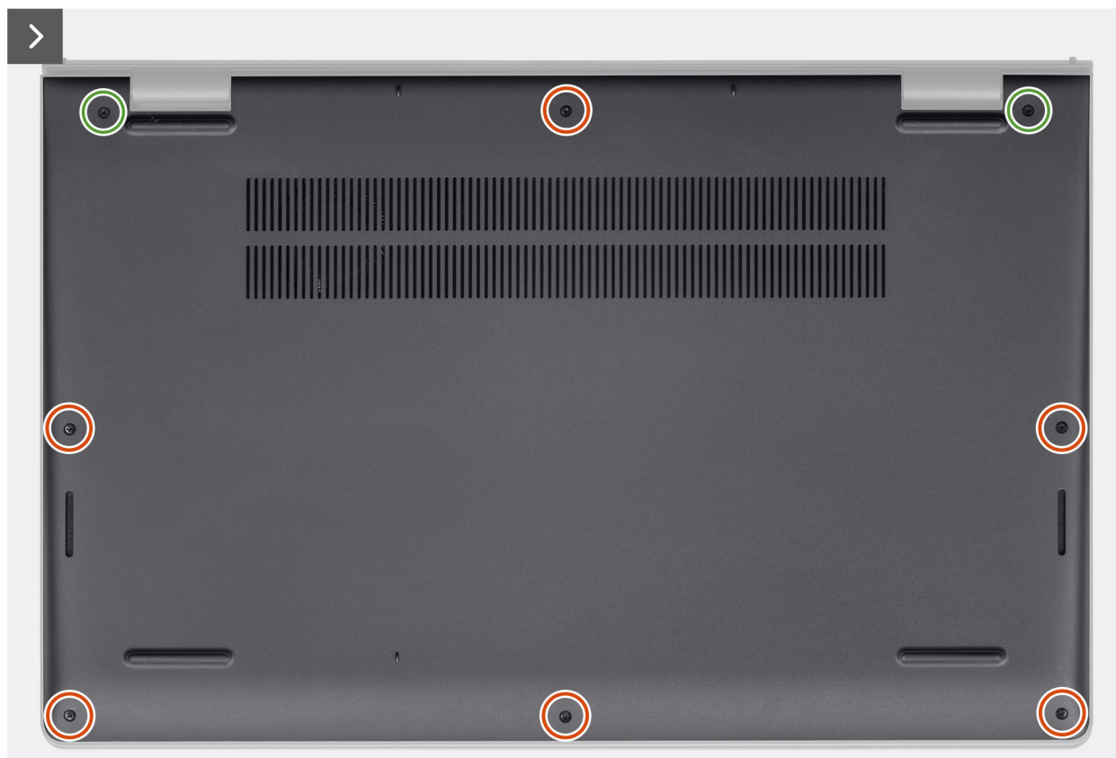
Figure 2. Removing the base cover
