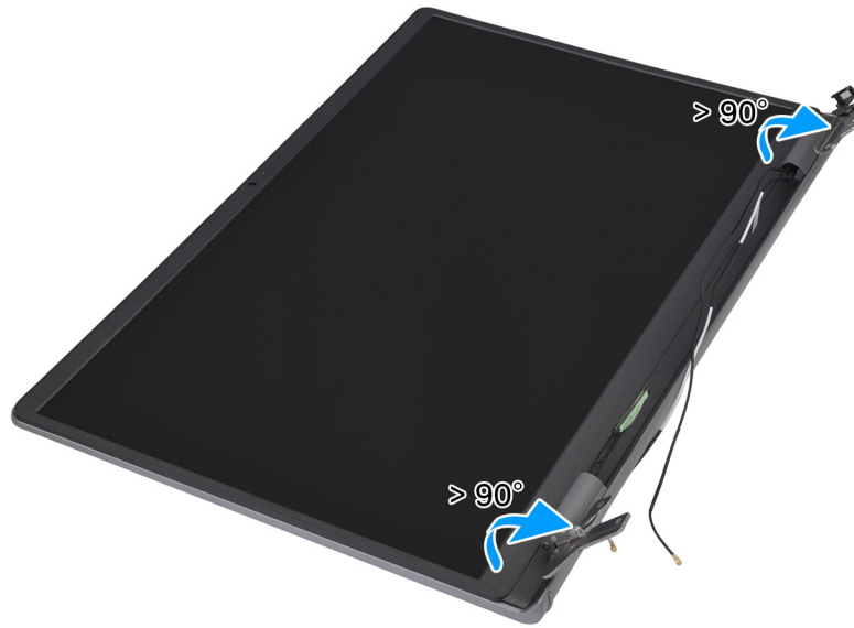
Figure 39. Opening the display hinges to at least 90 degrees
