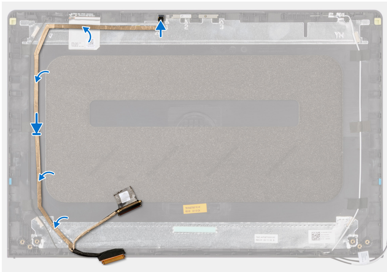
Figure 61. Installing the display cable
