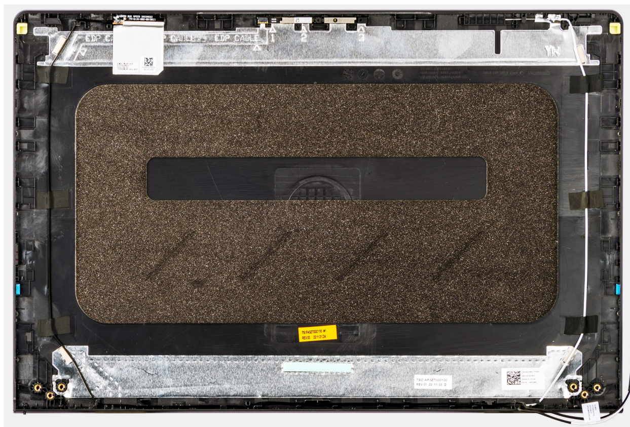
Figure 63. Installing the display back-cover and antenna assembly
