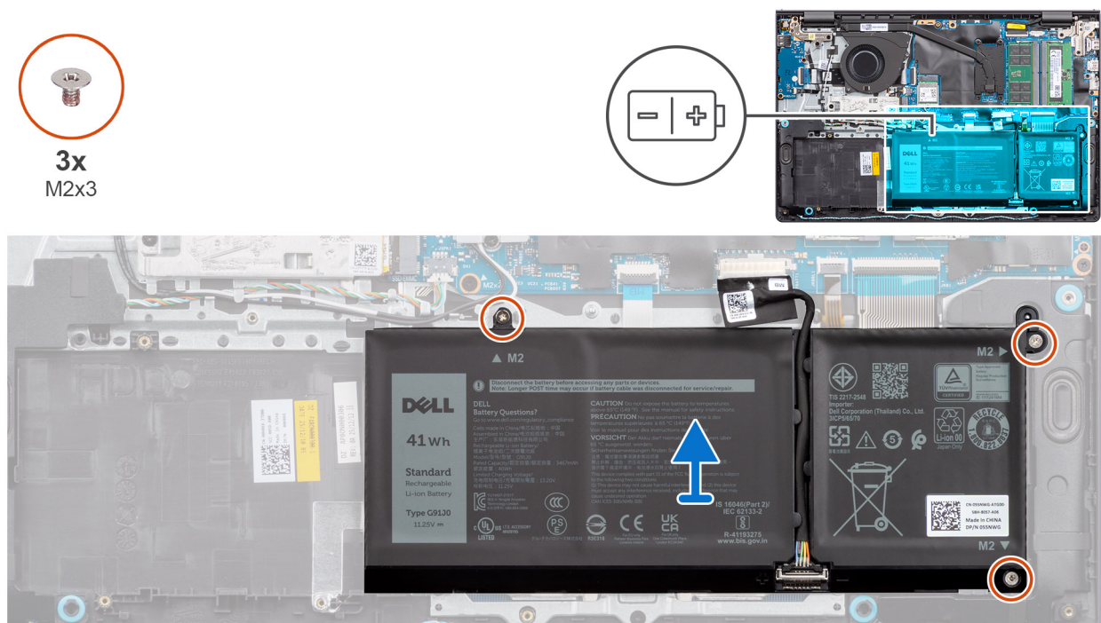
Figure 8. Removing the 3-cell battery
