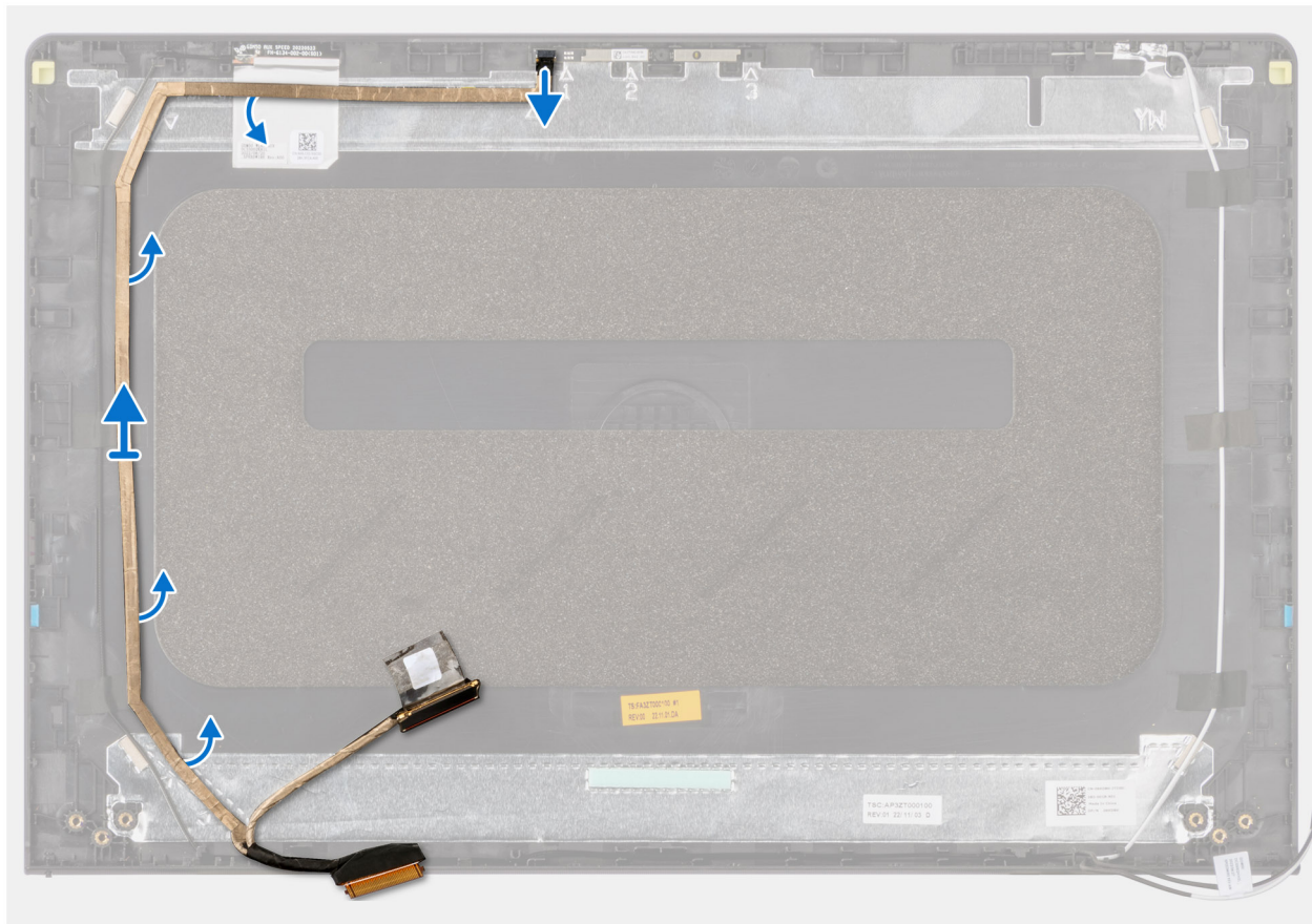
Figure 60. Removing the display cable
