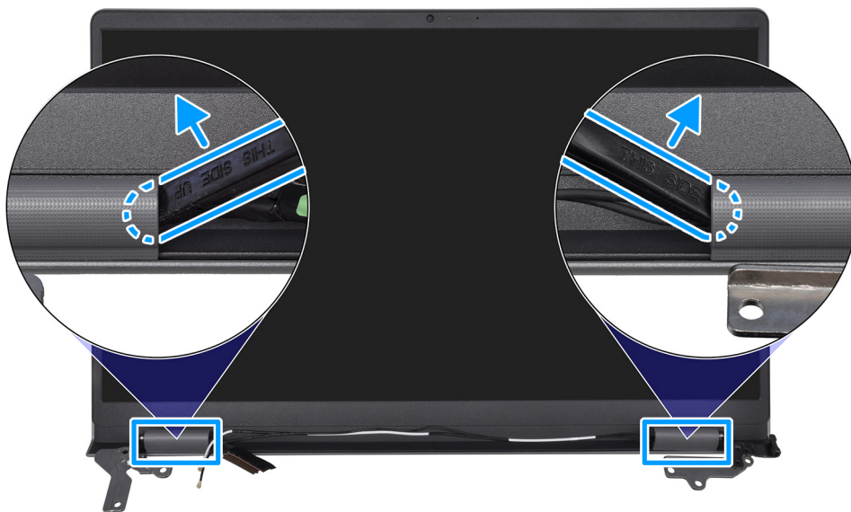
Figure 40. Prying the display hinges
