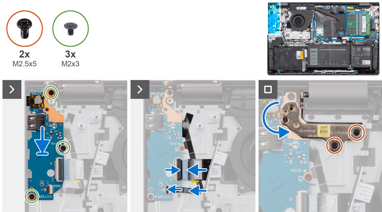
Figure 29. Installing I/O board
