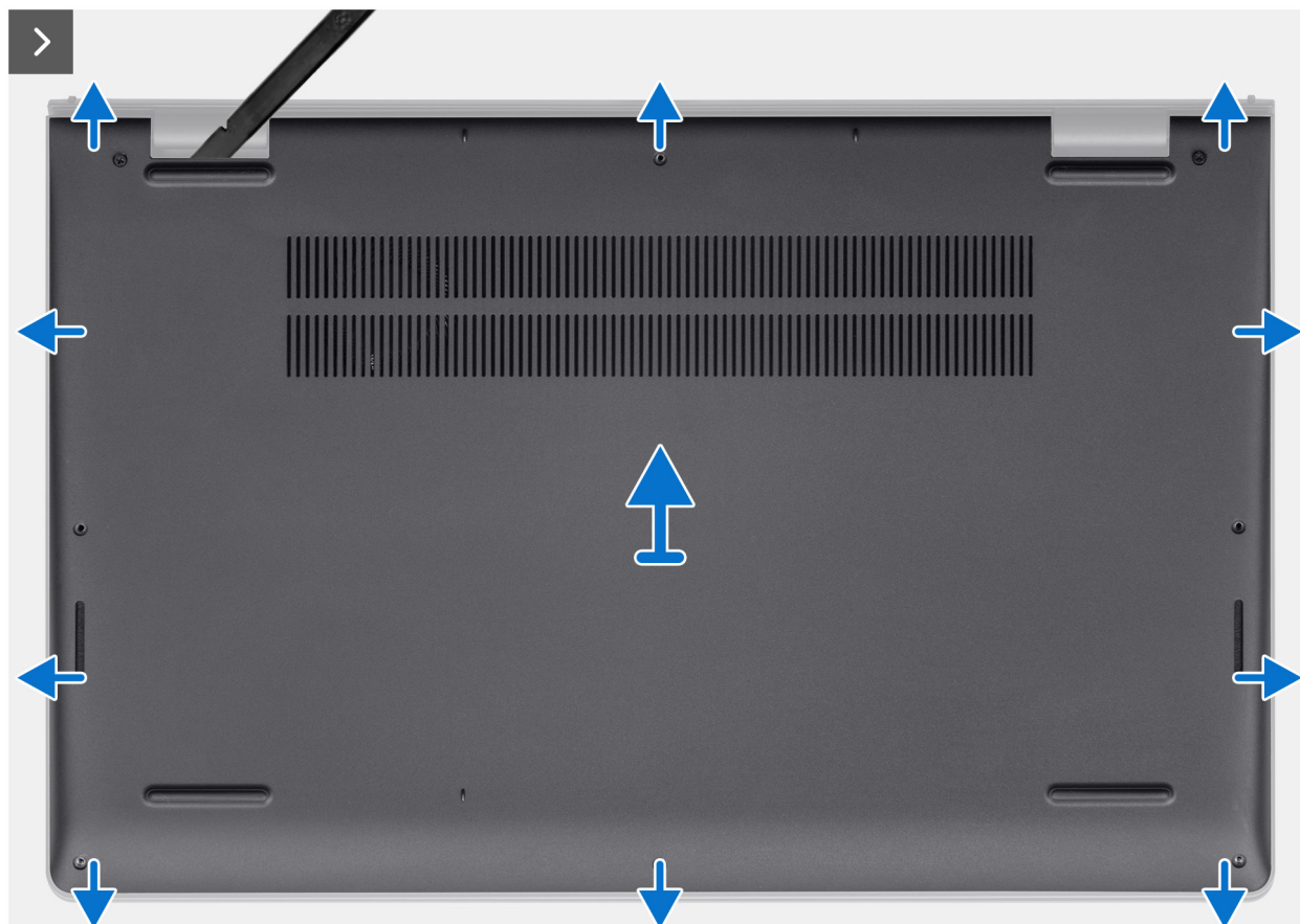
Figure 3. Removing the base cover
