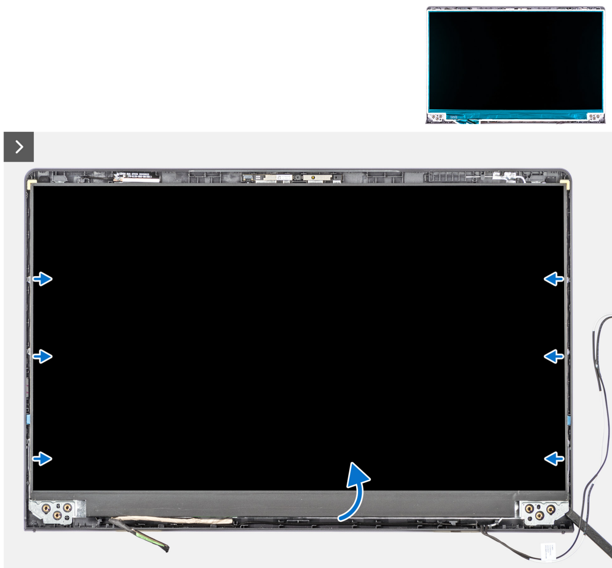
Figure 46. Removing the display panel
