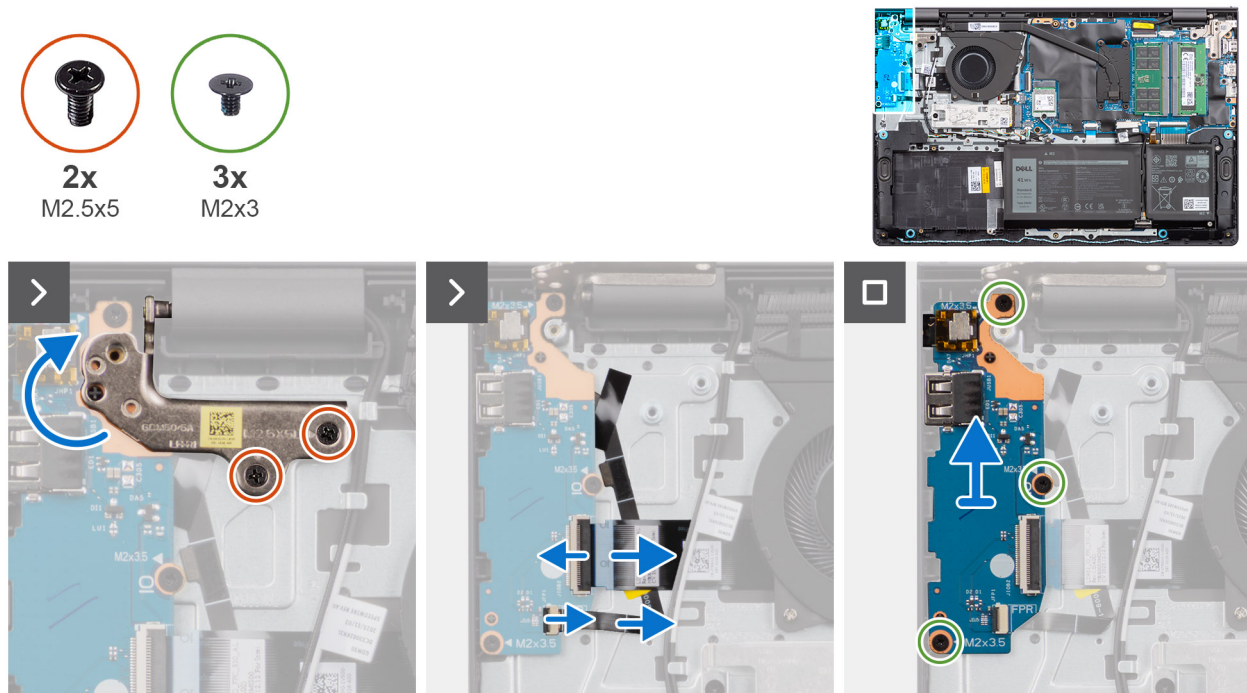
Figure 28. Removing the I/O board
