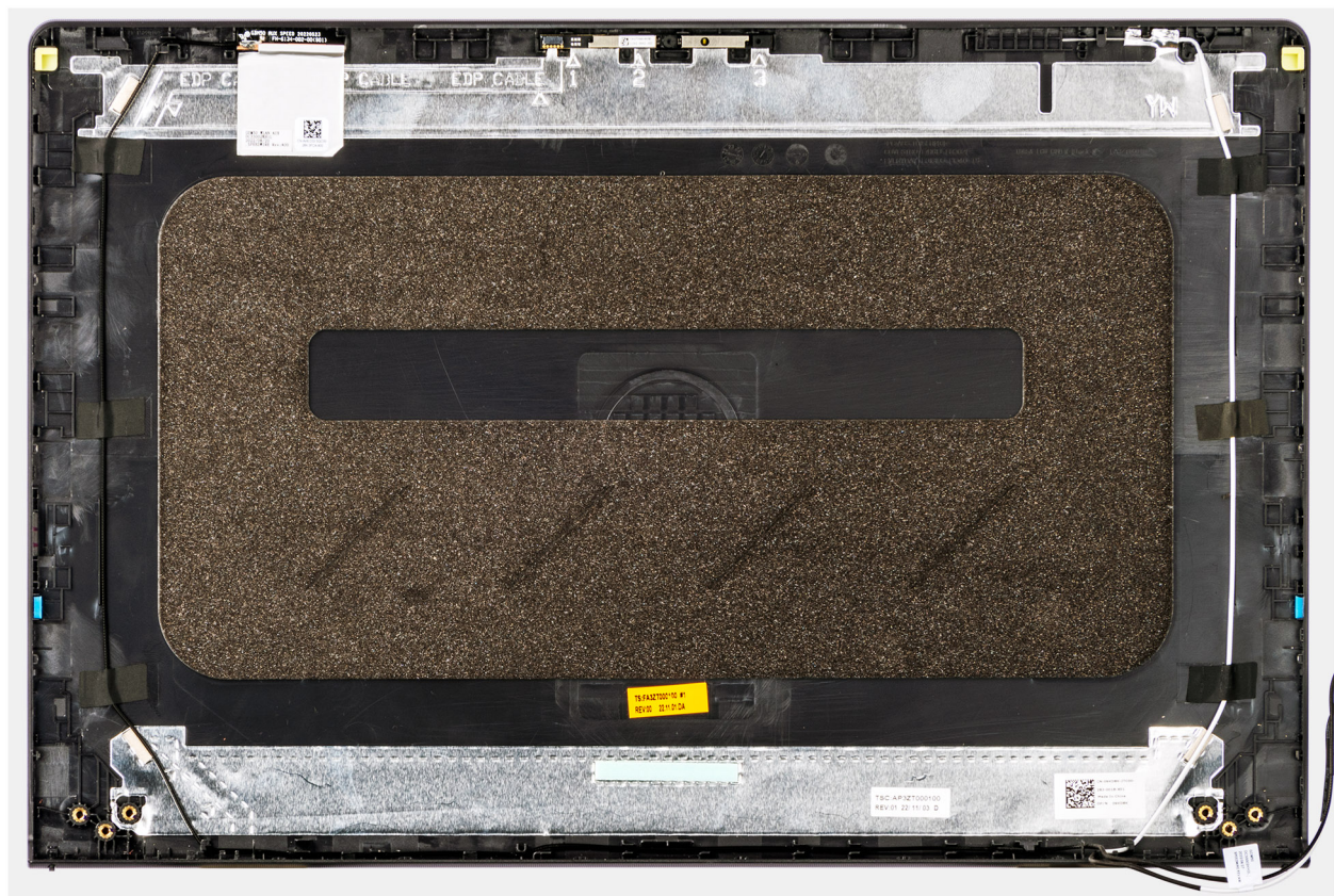
Figure 62. Removing the display back-cover and antenna assembly
