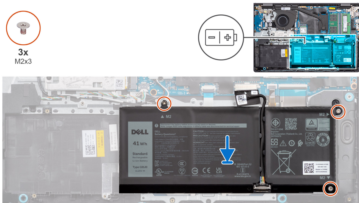
Figure 9. Installing the 3-cell battery
