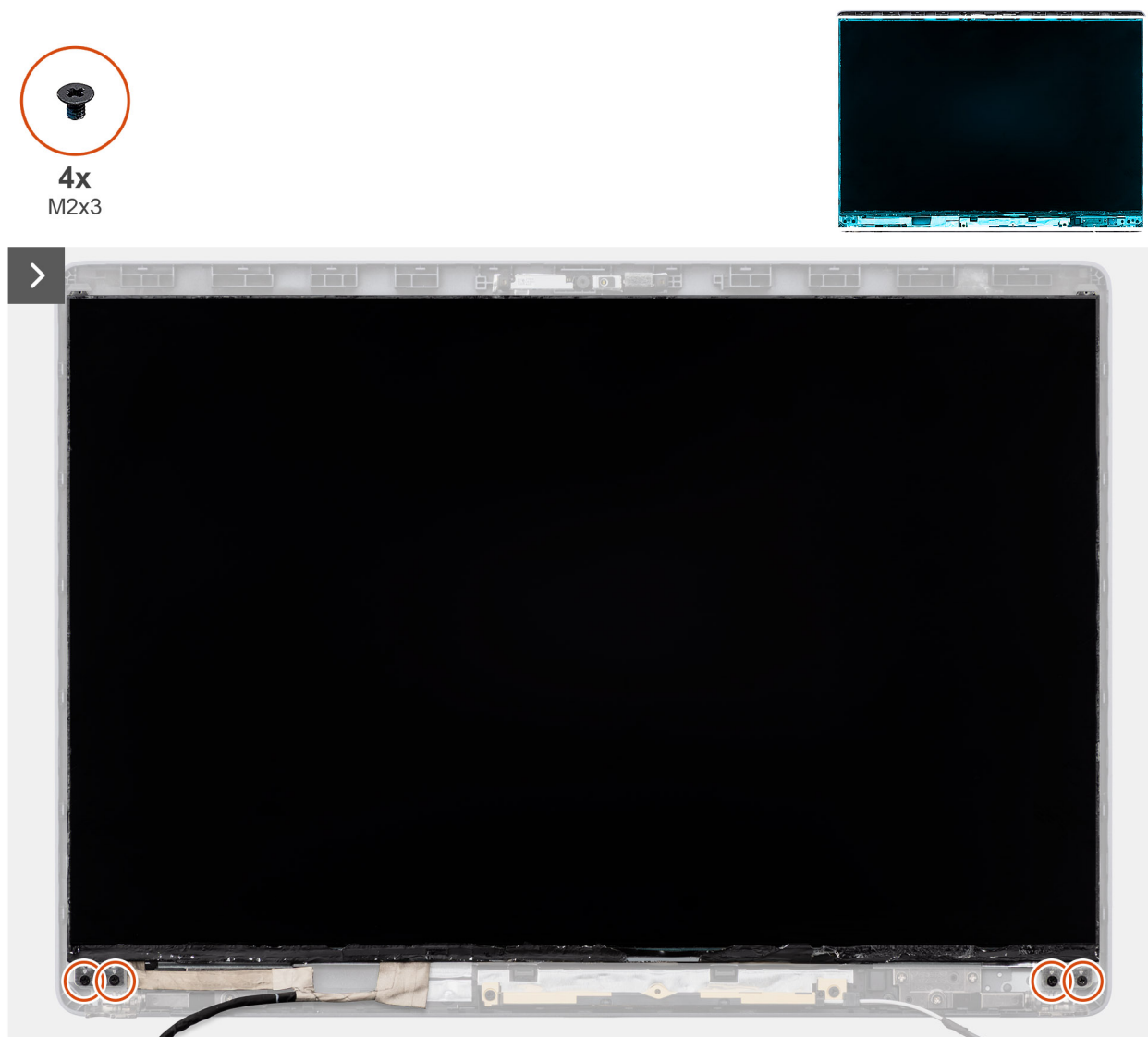
Figure 62. Removing the display panel
