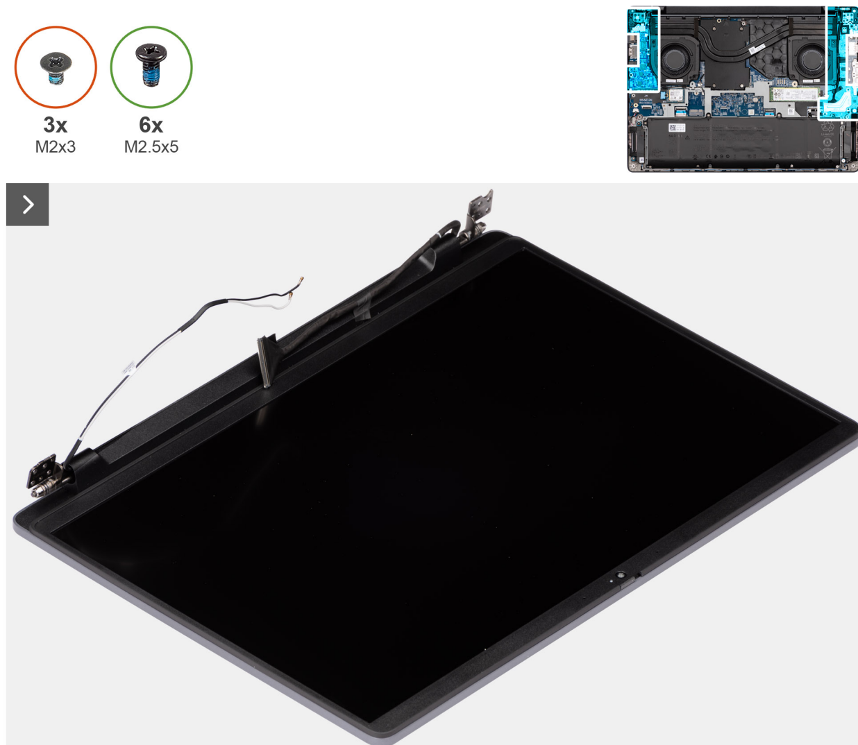
Figure 51. Installing the display assembly
