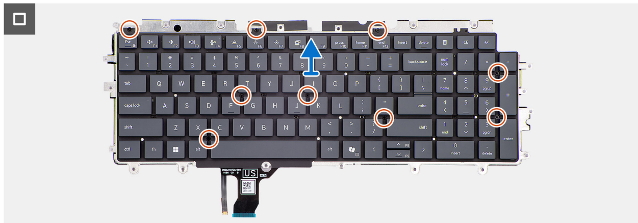
Figure 94. Removing the keyboard
