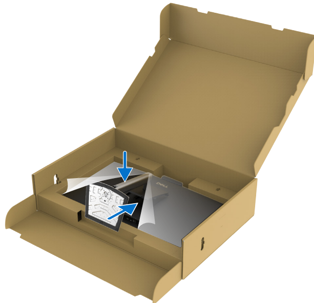
Figure 17. Insert the tabs on the stand riser into the slots
