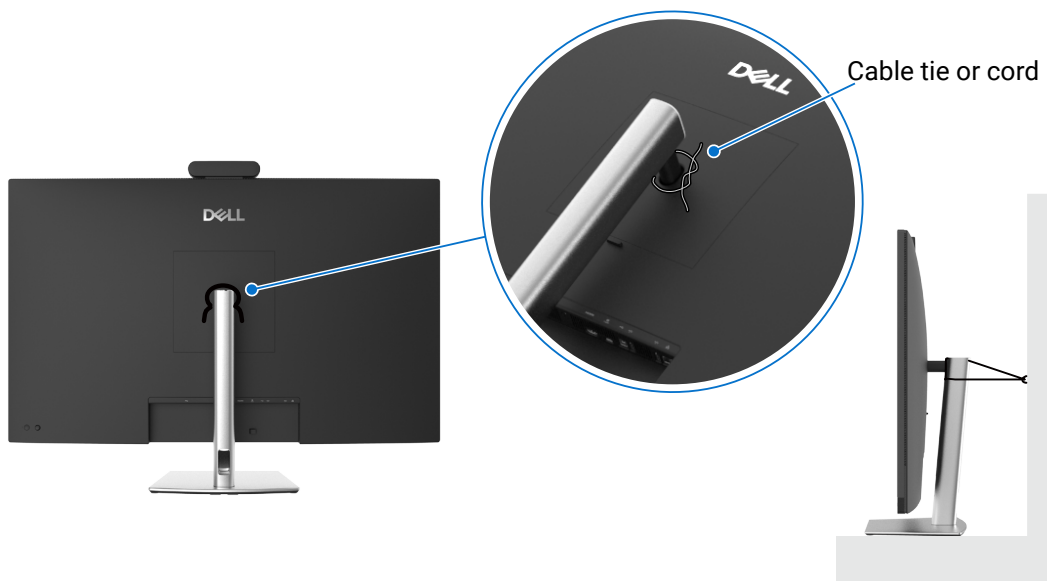
Figure 26. Prevent the monitor from falling
