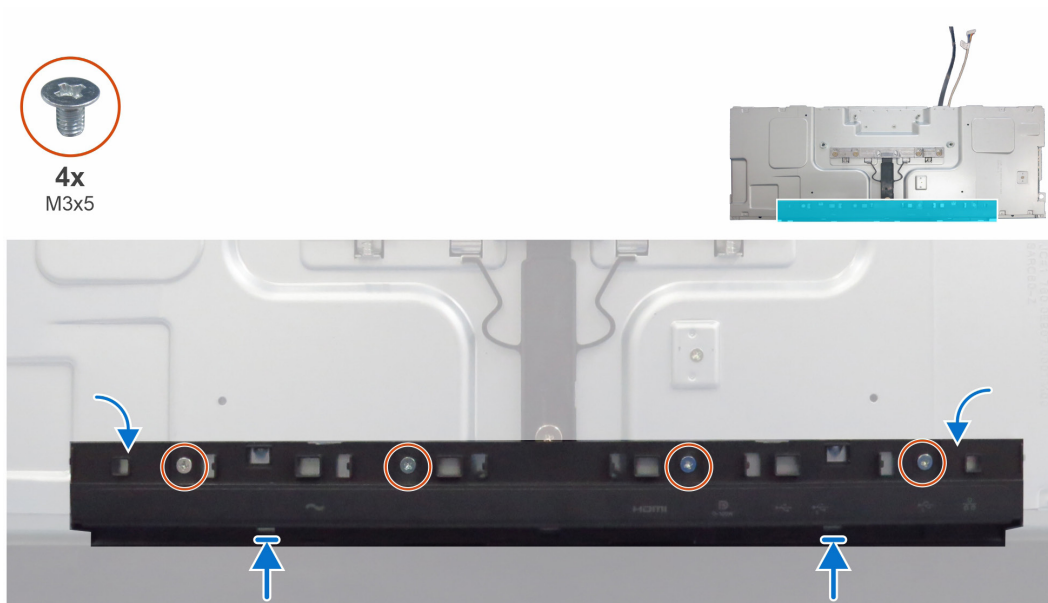
Figure 14. Installing the I/O cover
