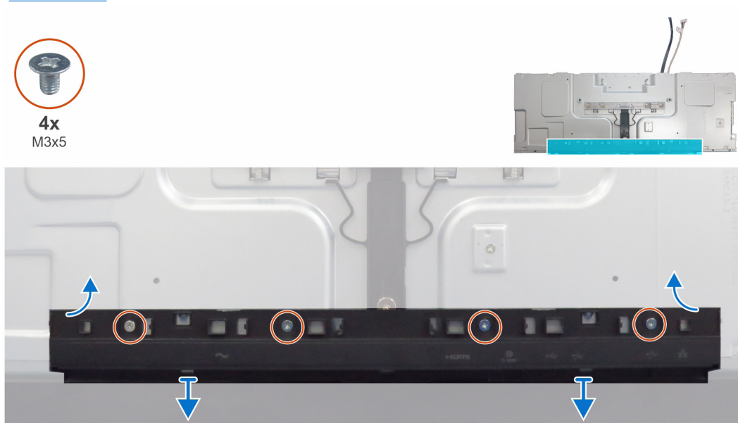
Figure 13. Removing the I/O cover
