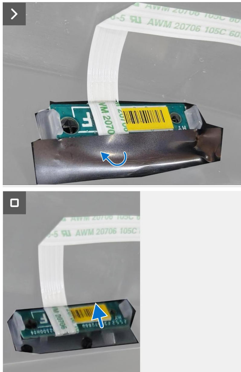
Figure 13. Removing the LED board
