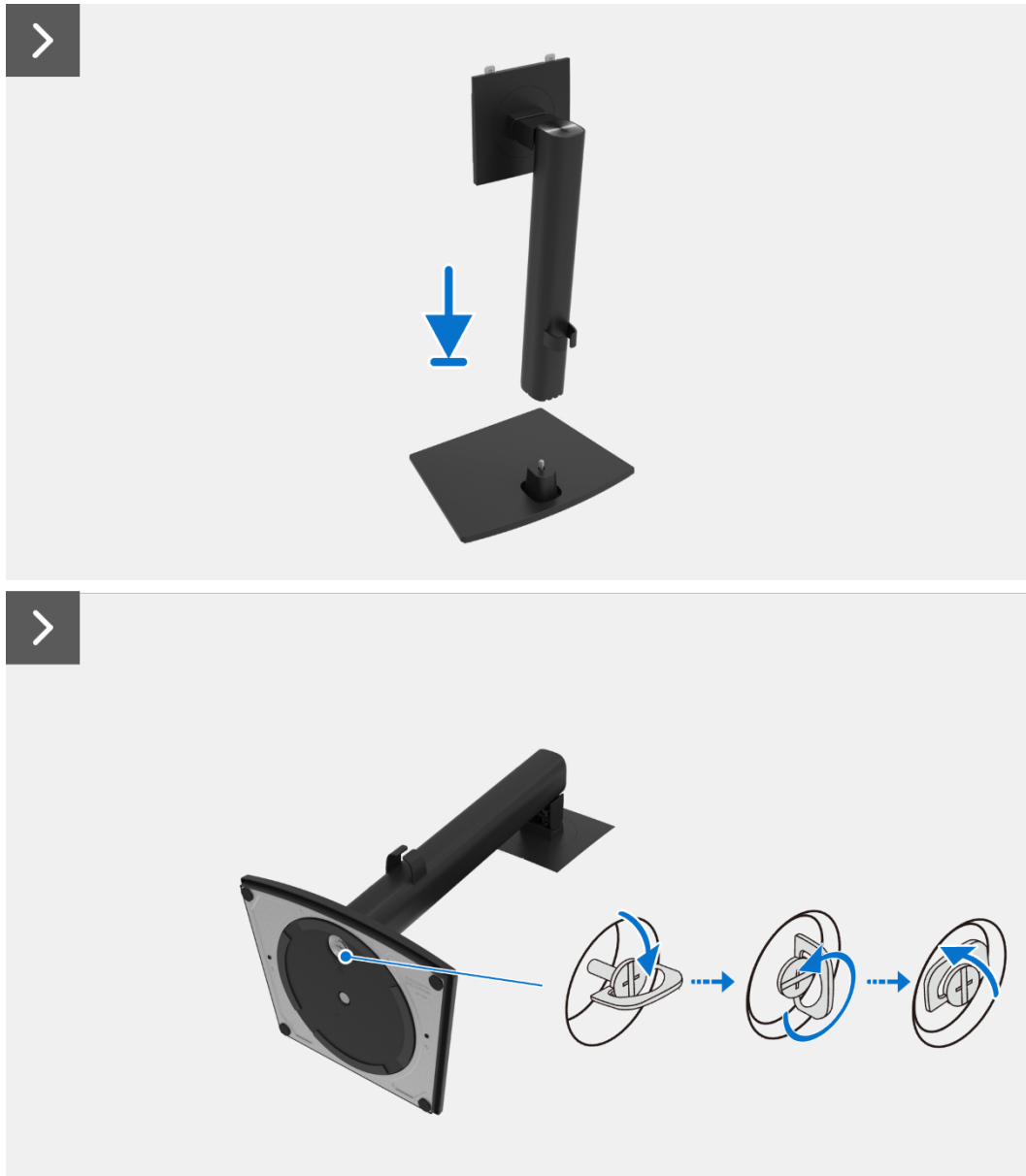
Figure 3. Installing the stand
