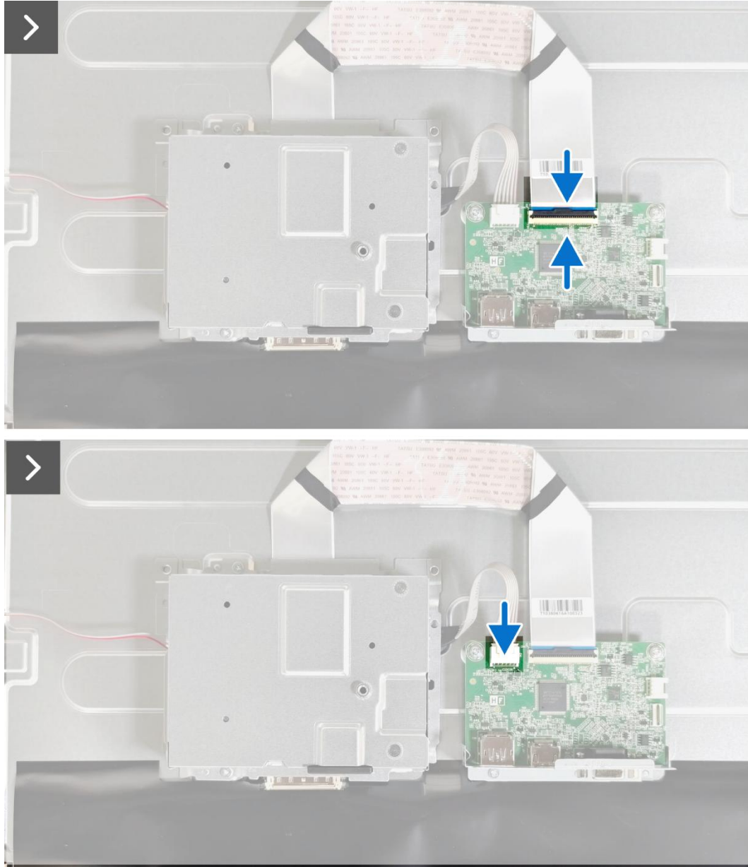
Figure 24. Installing the chassis assembly
