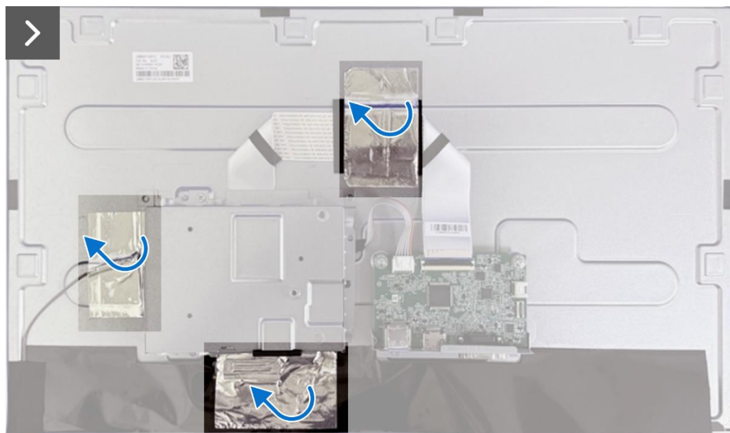
Figure 20. Removing the chassis assembly
