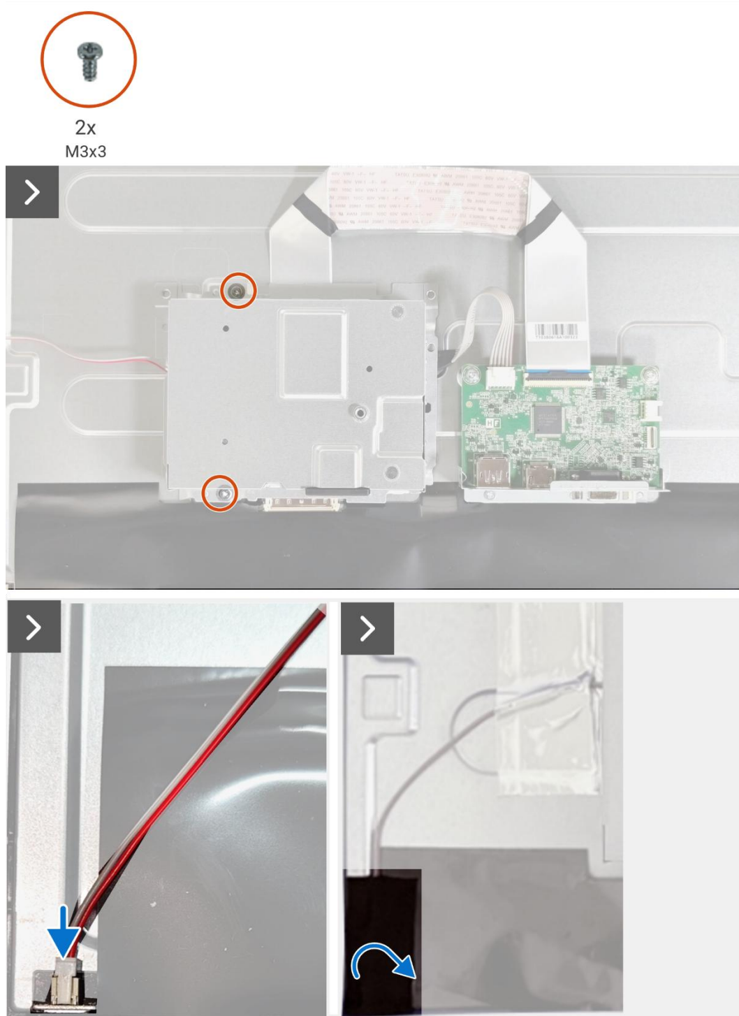
Figure 25. Installing the chassis assembly
