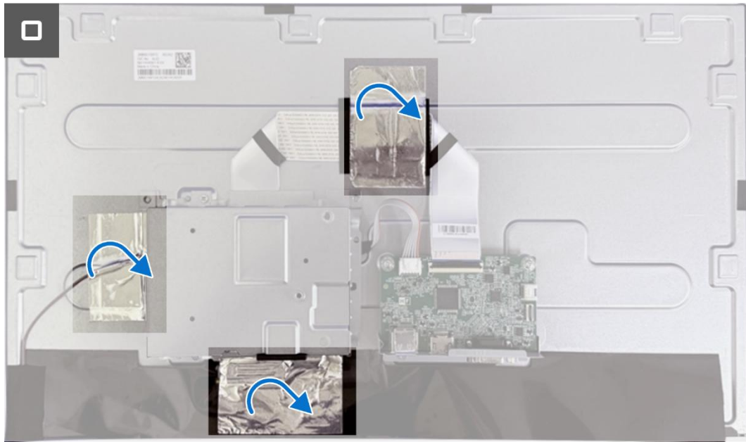
Figure 26. Installing the chassis assembly
