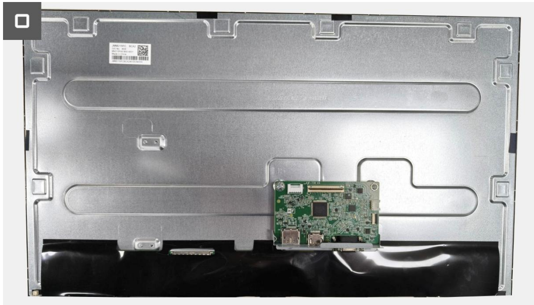
Figure 23. Removing the chassis assembly
