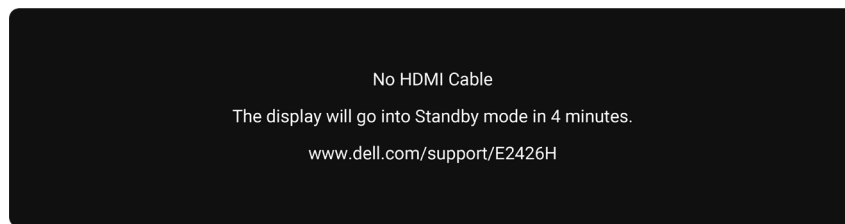
Figure 36. HDMI cable disconnected warning message
