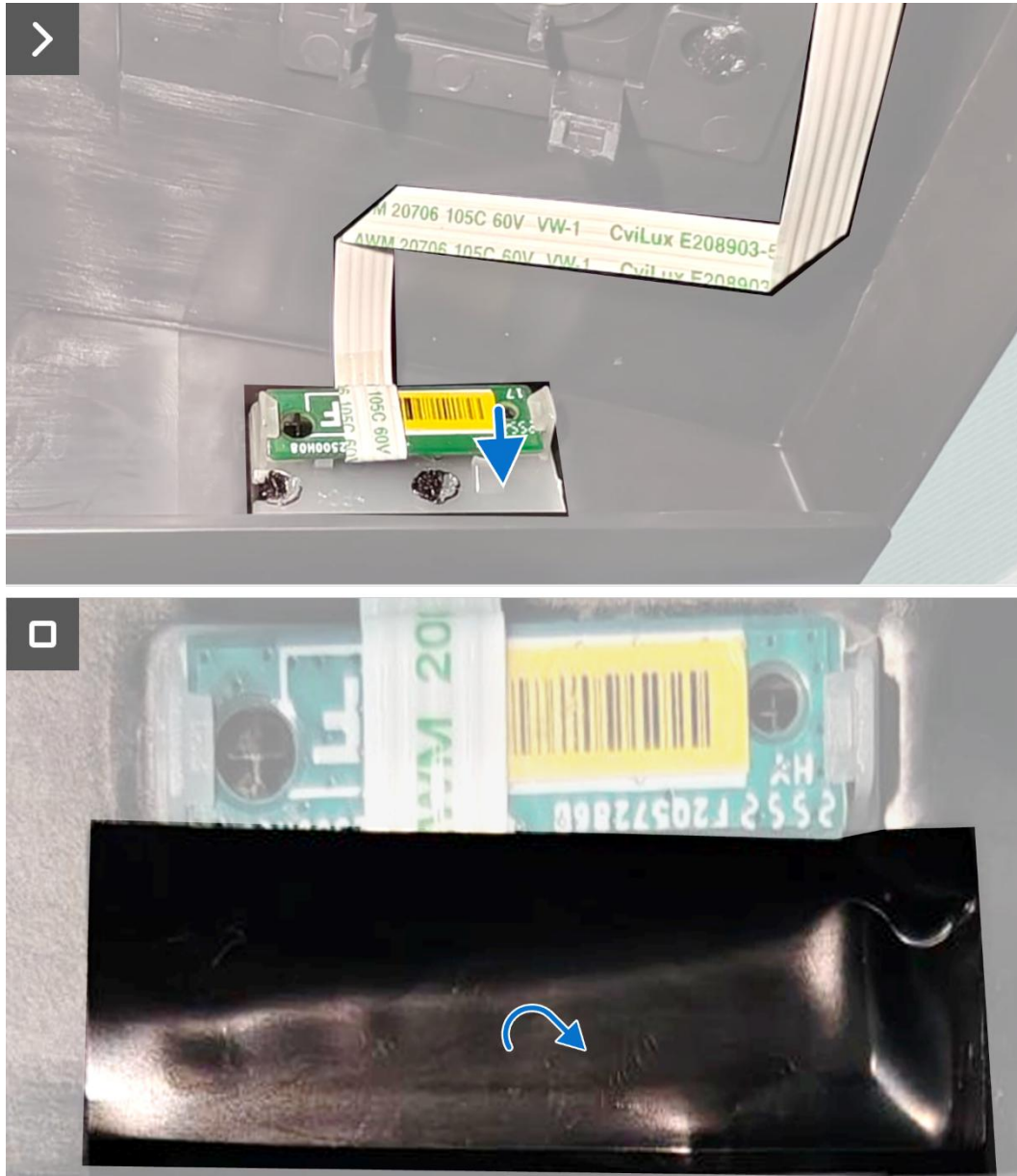
Figure 12. Installing the LED board
