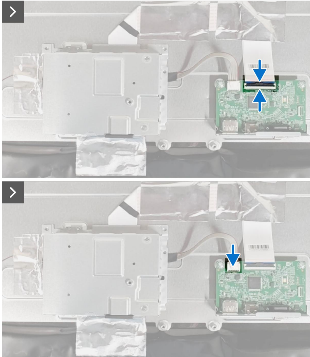
Figure 17. Installing the chassis assembly
