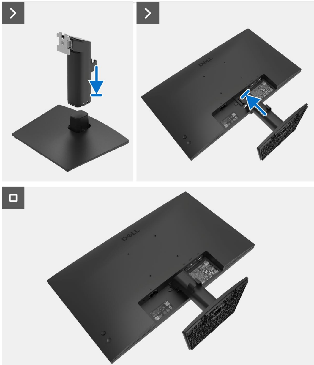
Figure 2. Installing the stand
