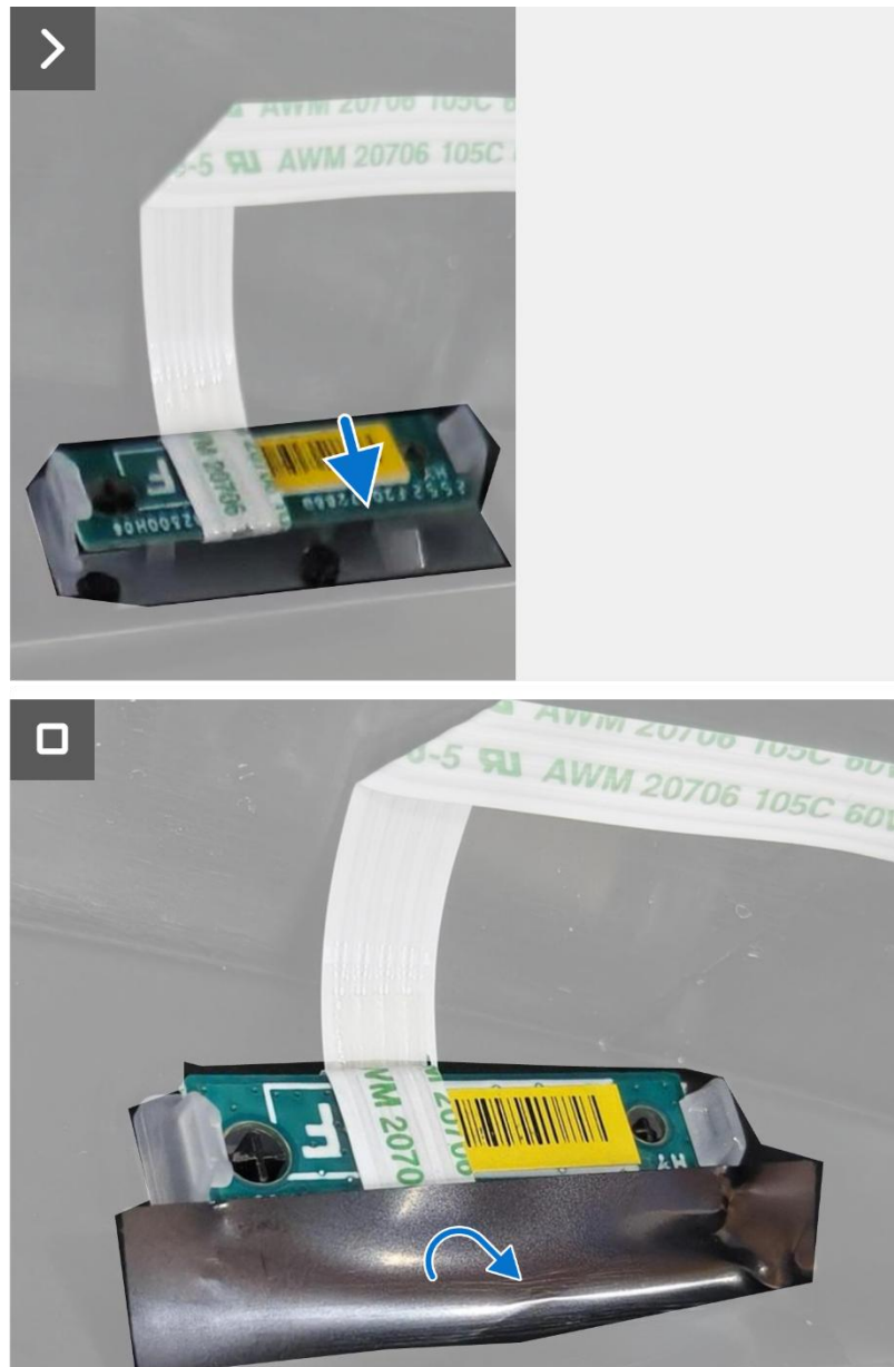
Figure 14. Installing the LED board
