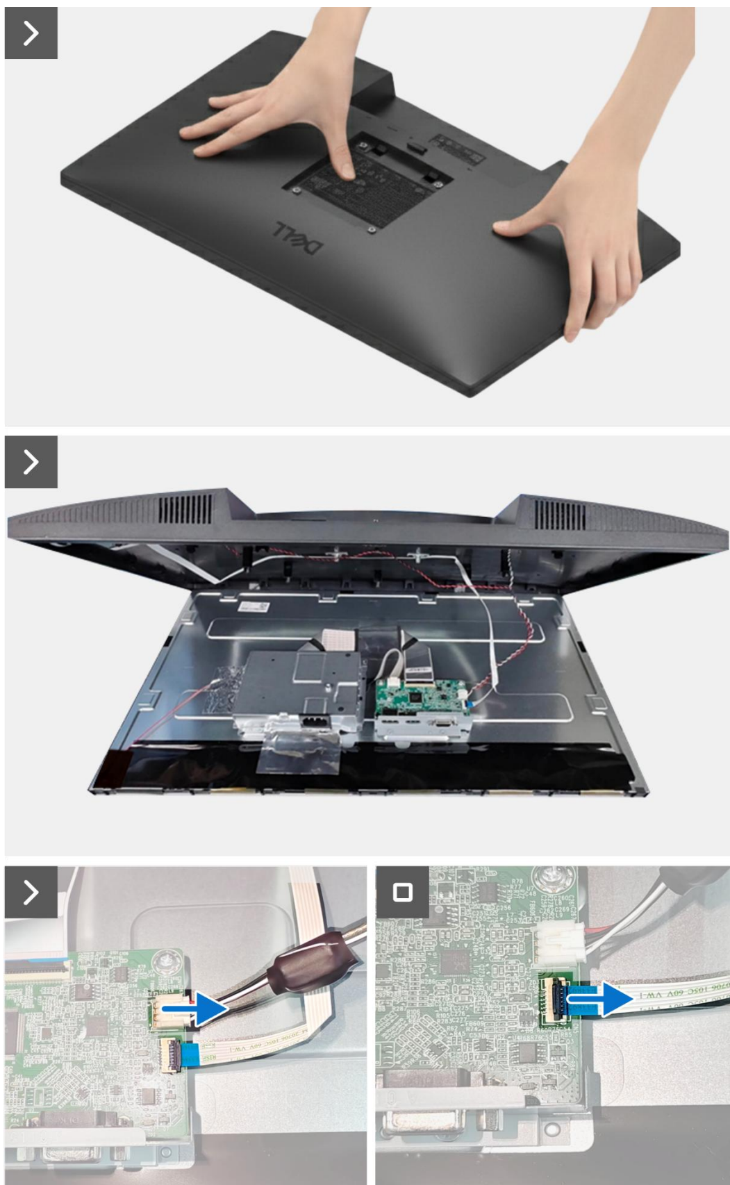
Figure 6. Removing the back cover
