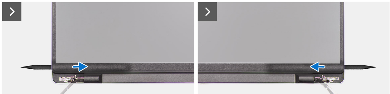
Figure 52. Removing the display bezel
