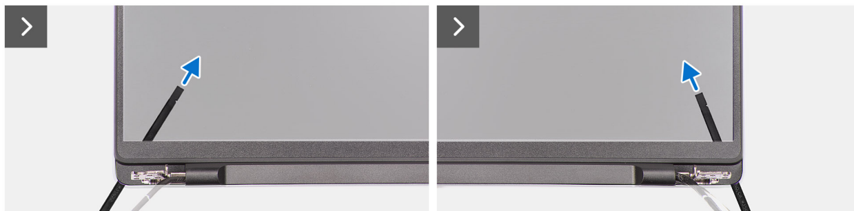
Figure 49. Removing the display bezel
