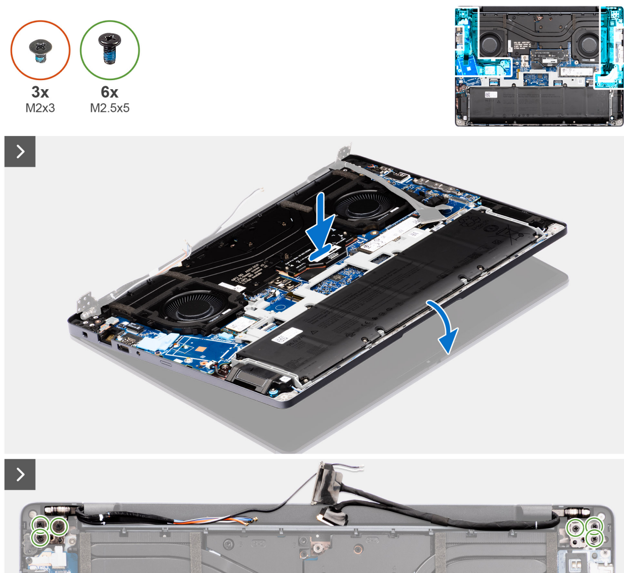
Figure 46. Installing the display assembly
