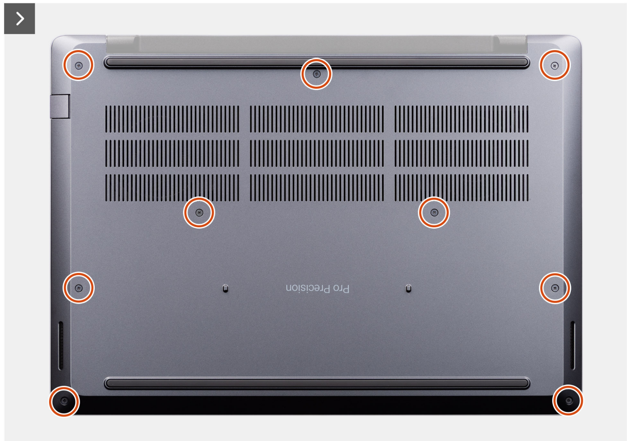
Figure 2. Loosen the captive screws
