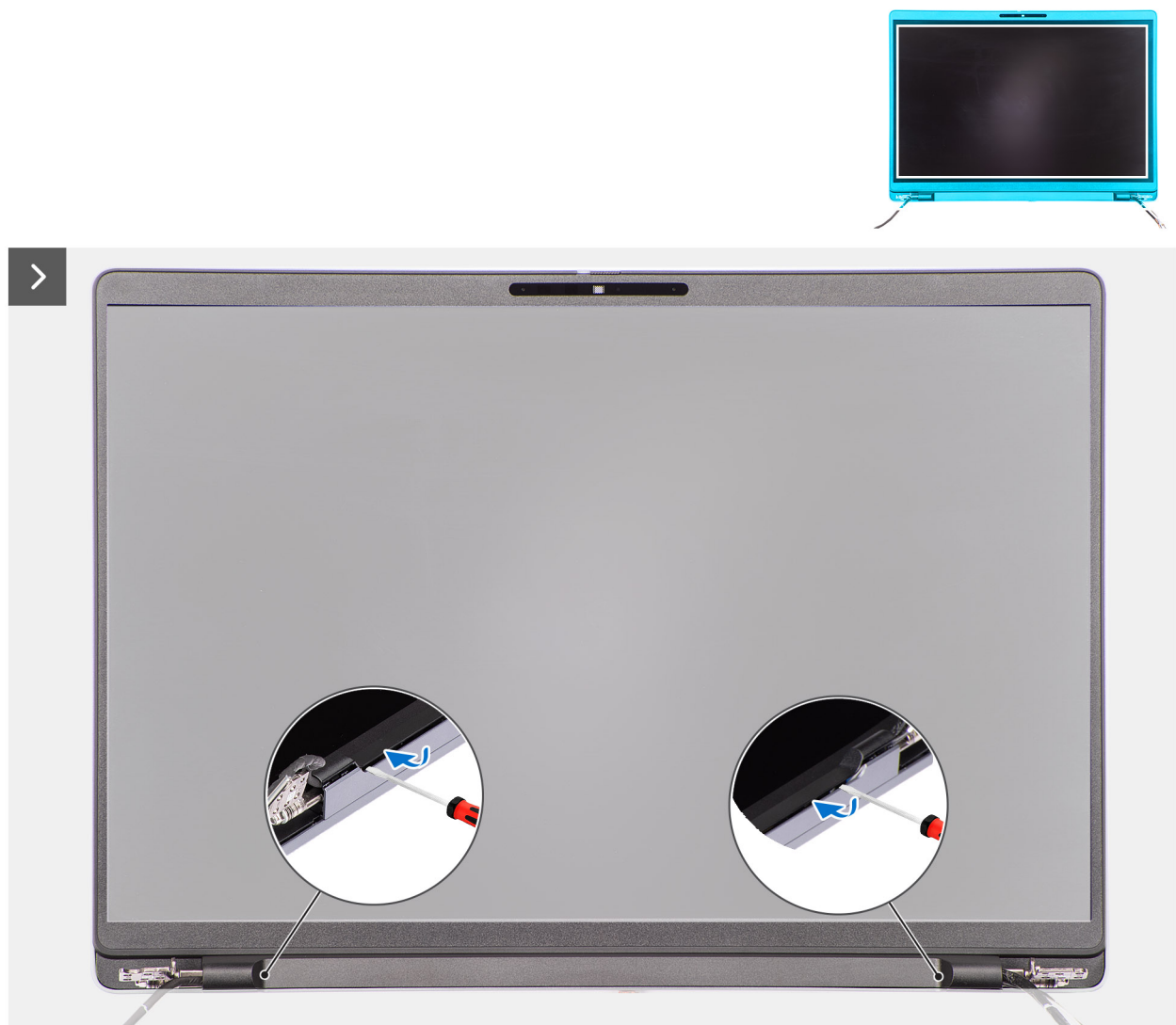
Figure 48. Removing the display bezel
