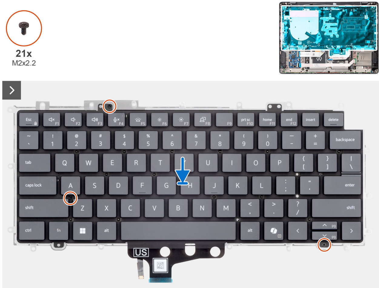
Figure 80. Installing the keyboard
