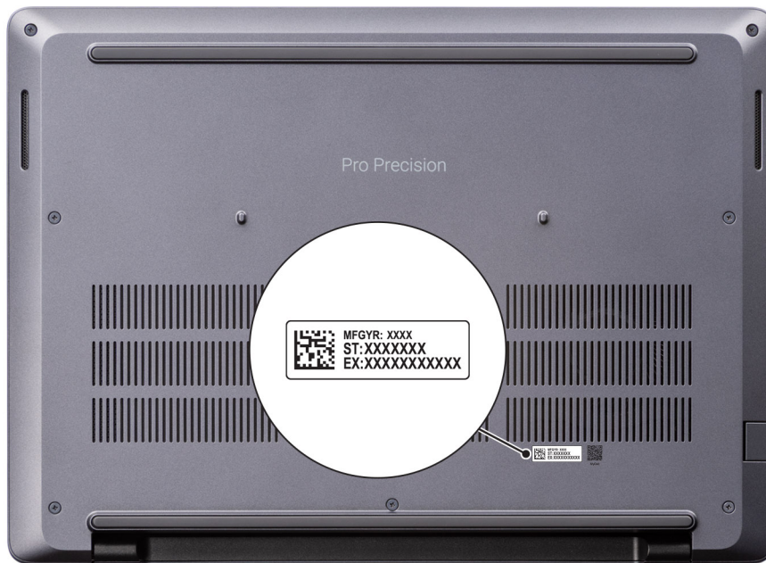
Figure 7. Service Tag/Express Service Code location
