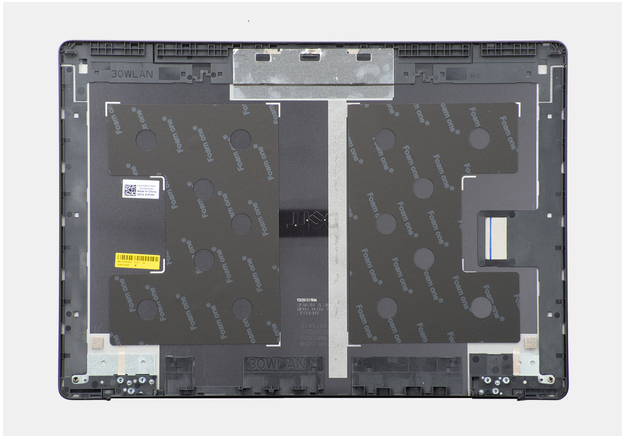
Figure 58. Removing the display-back cover
