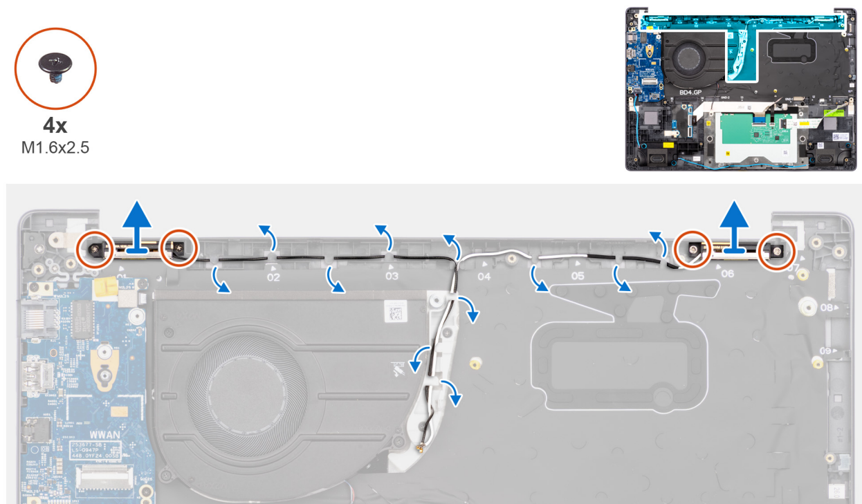
Figure 69. Removing the wireless-antenna modules
