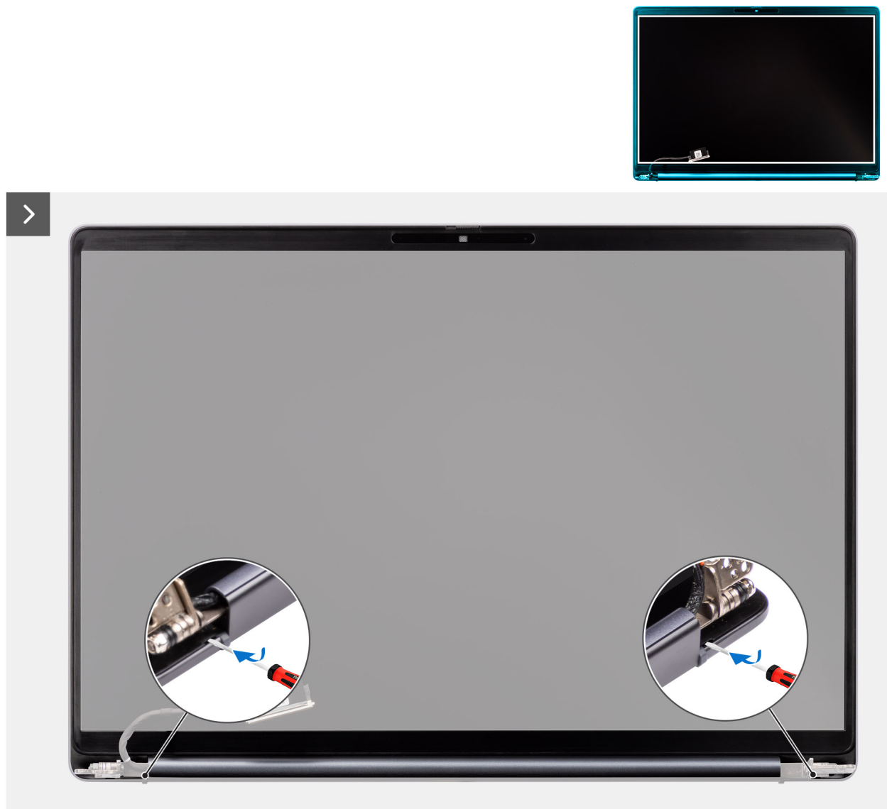
Figure 43. Removing the display bezel
