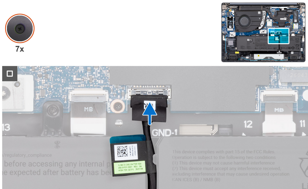
Figure 7. Connecting the battery cable
