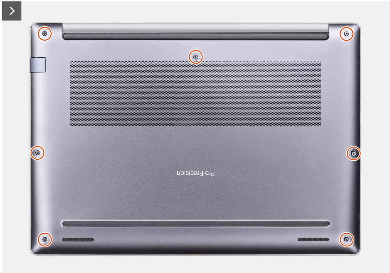
Figure 4. Removing the base cover
