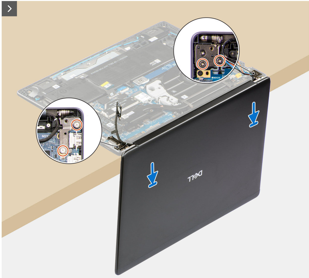
Figure 41. Installing the display assembly
