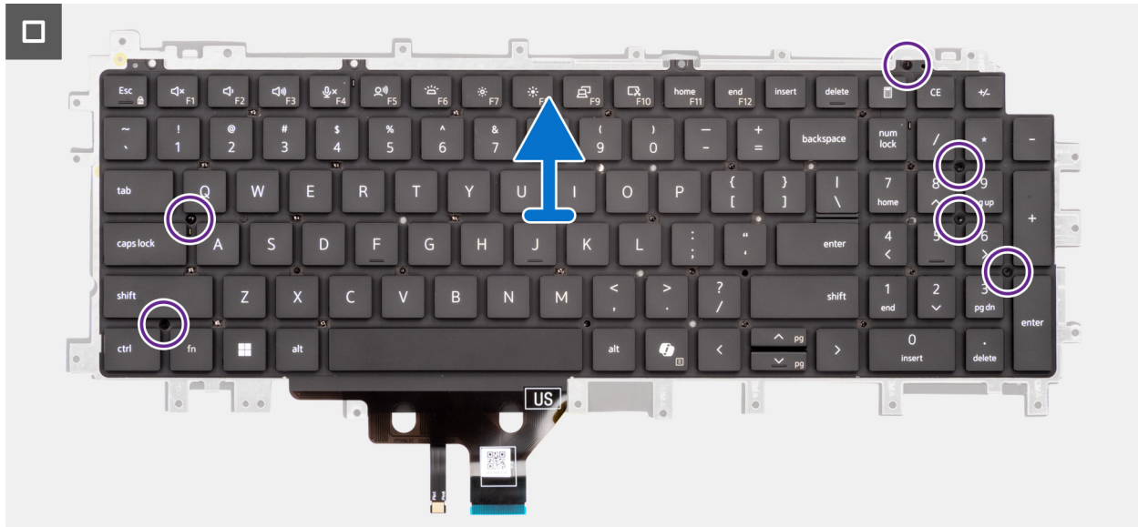
Figure 72. Removing the keyboard
