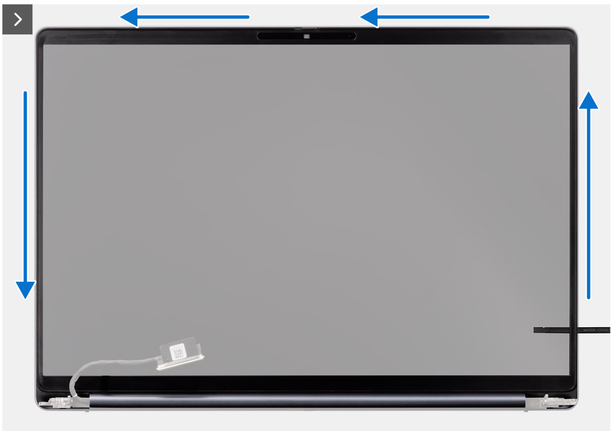
Figure 45. Removing the display bezel
