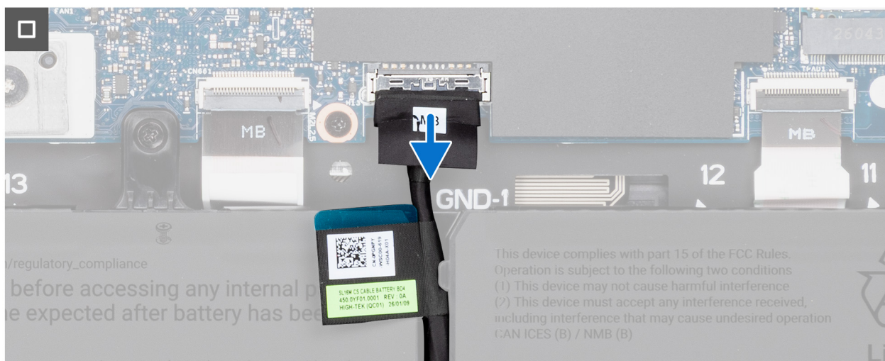
Figure 6. Disconnecting the battery cable
