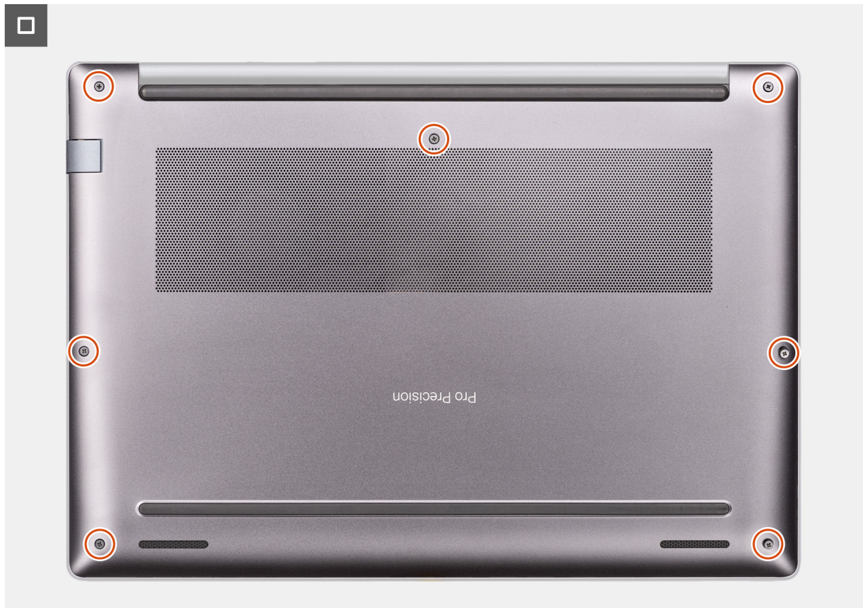
Figure 9. Installing the base cover
