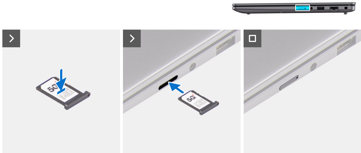
Figure 3. Installing the nano-SIM card tray
