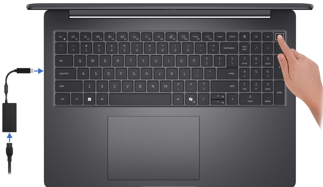
Figure 7. Connect the power adapter and press the power button
