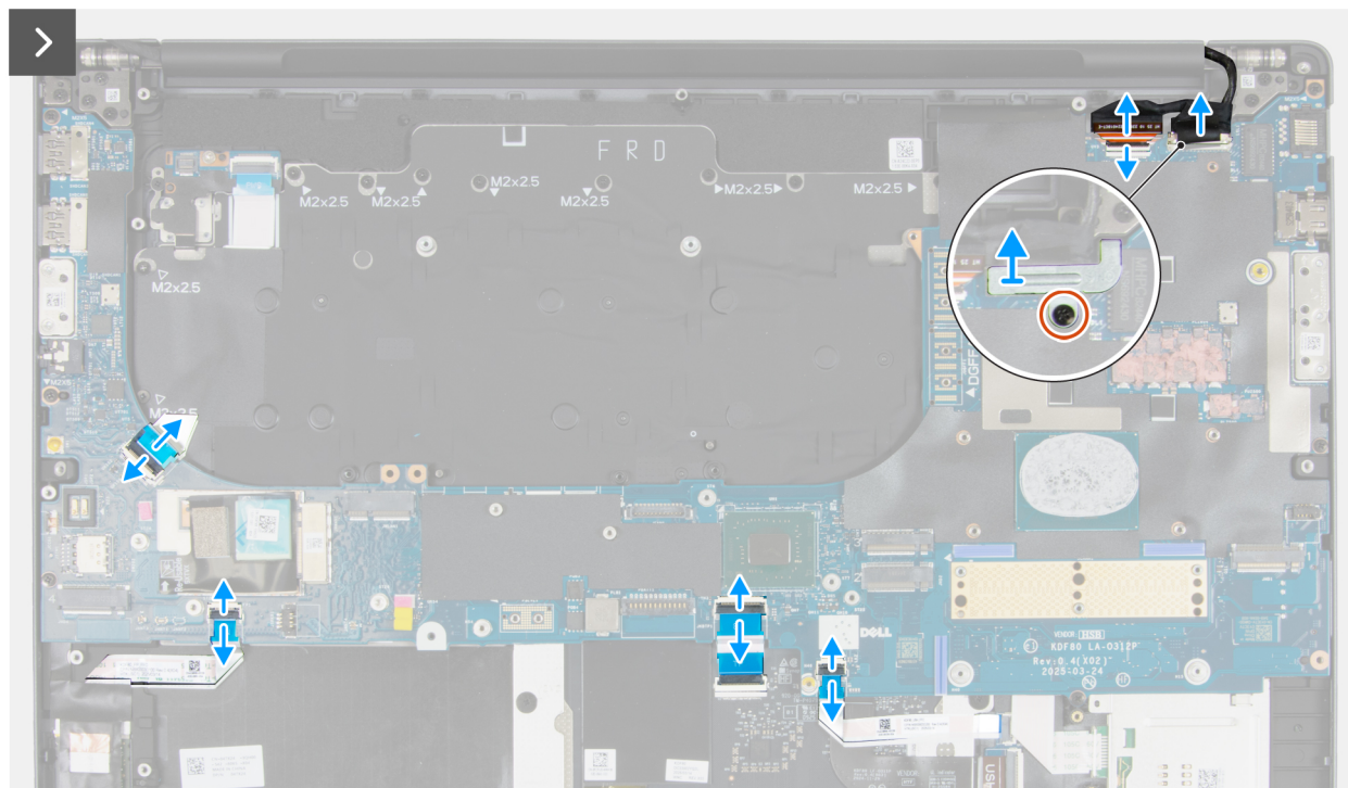
Figure 107. Removing the system board
