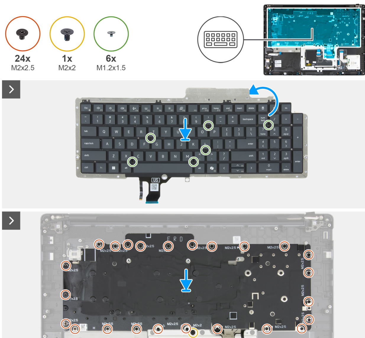
Figure 119. Installing the keyboard
