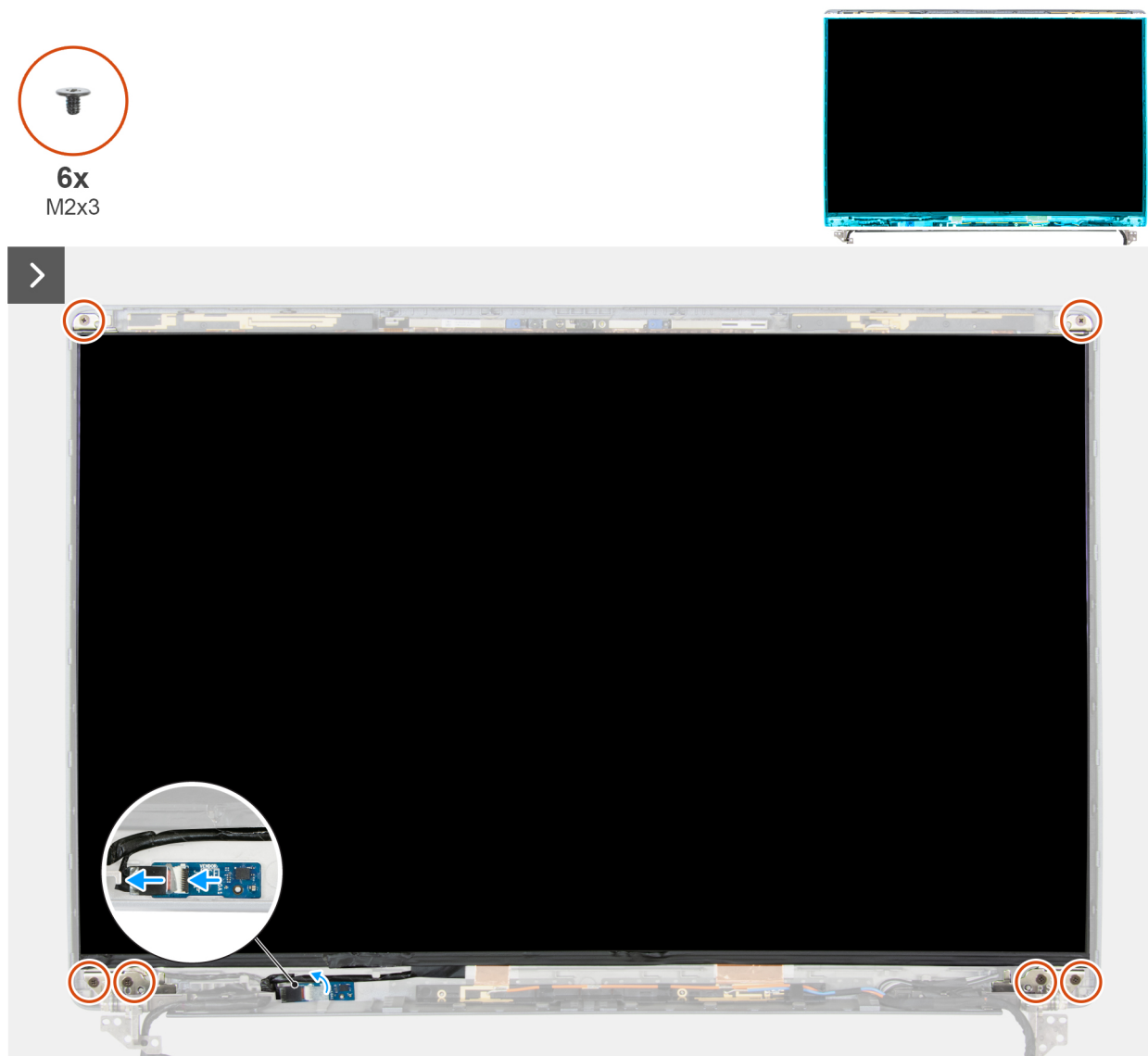
Figure 95. Removing the display panel
