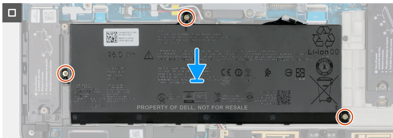
Figure 47. Replacing the battery
