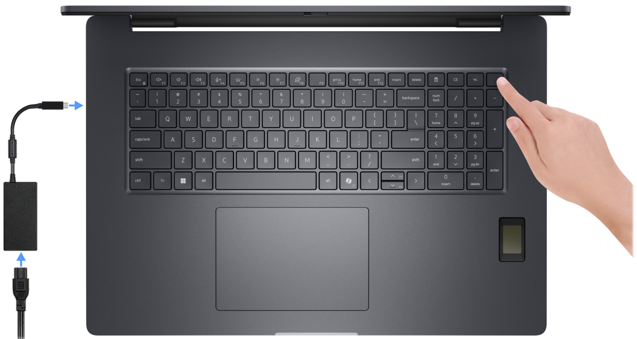
Figure 7. Connect the power adapter and press the power button.
