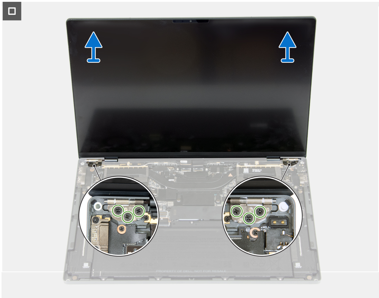
Figure 18. Removing the display assembly
