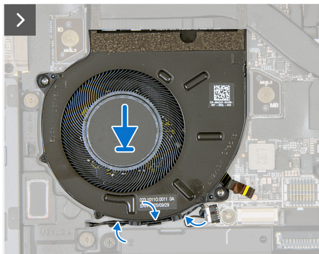
Figure 22. Installing the left-thermal fan
