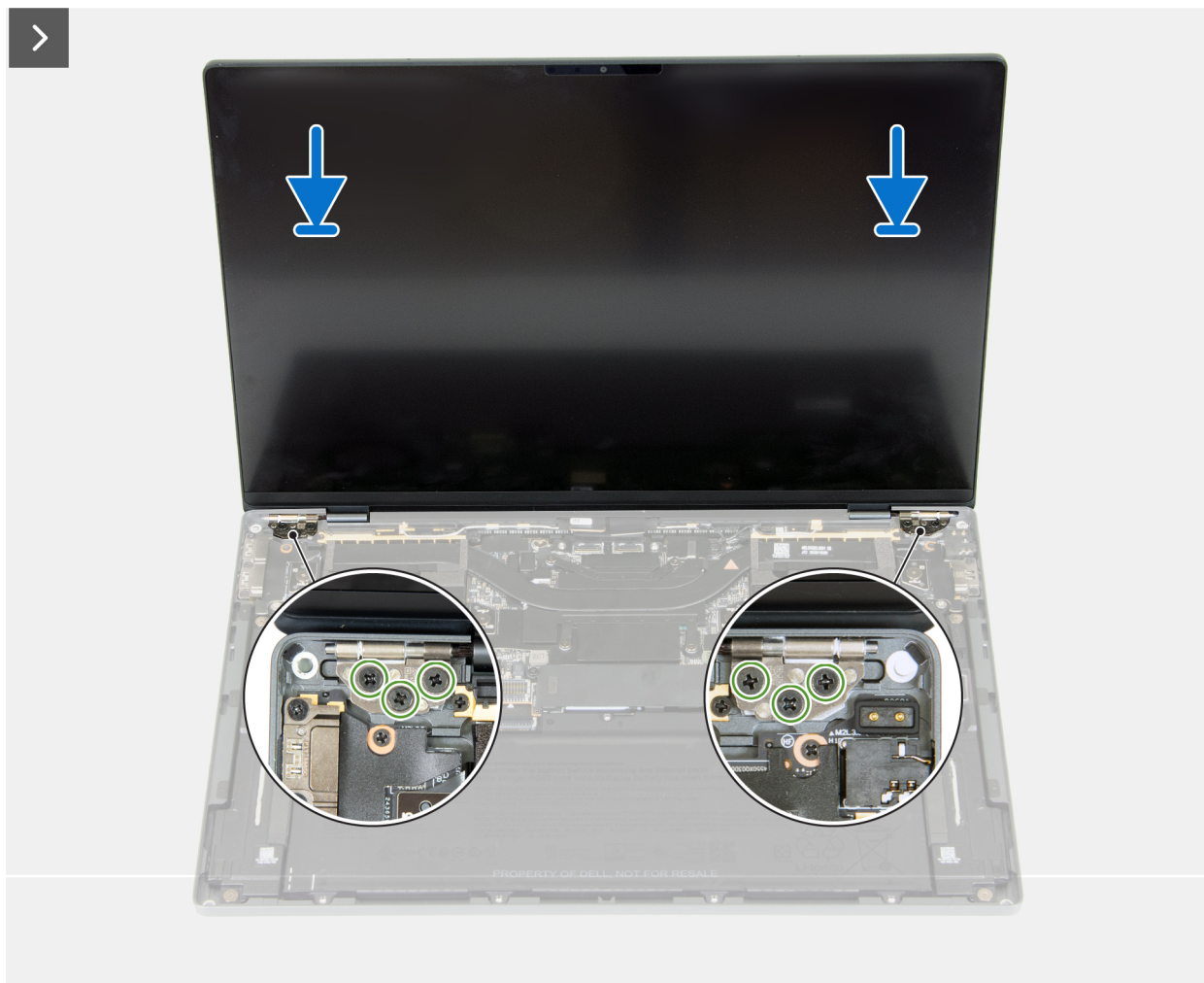
Figure 19. Installing the display assembly
