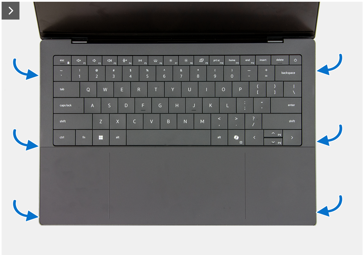
Figure 3. Loosen the palm-rest and keyboard assembly from the base cover
