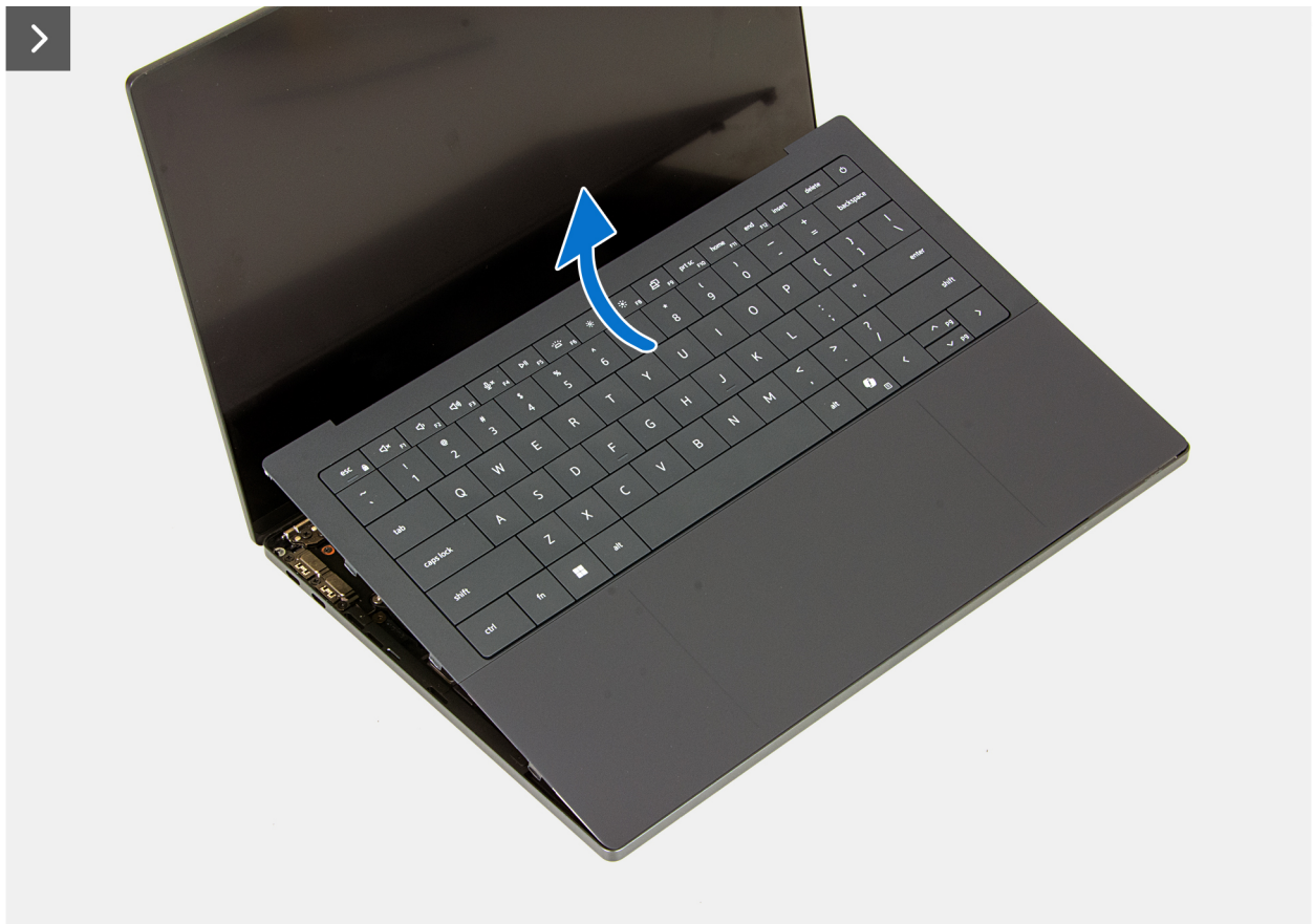
Figure 4. Carefully lift the palm-rest and keyboard assembly away from the base cover
