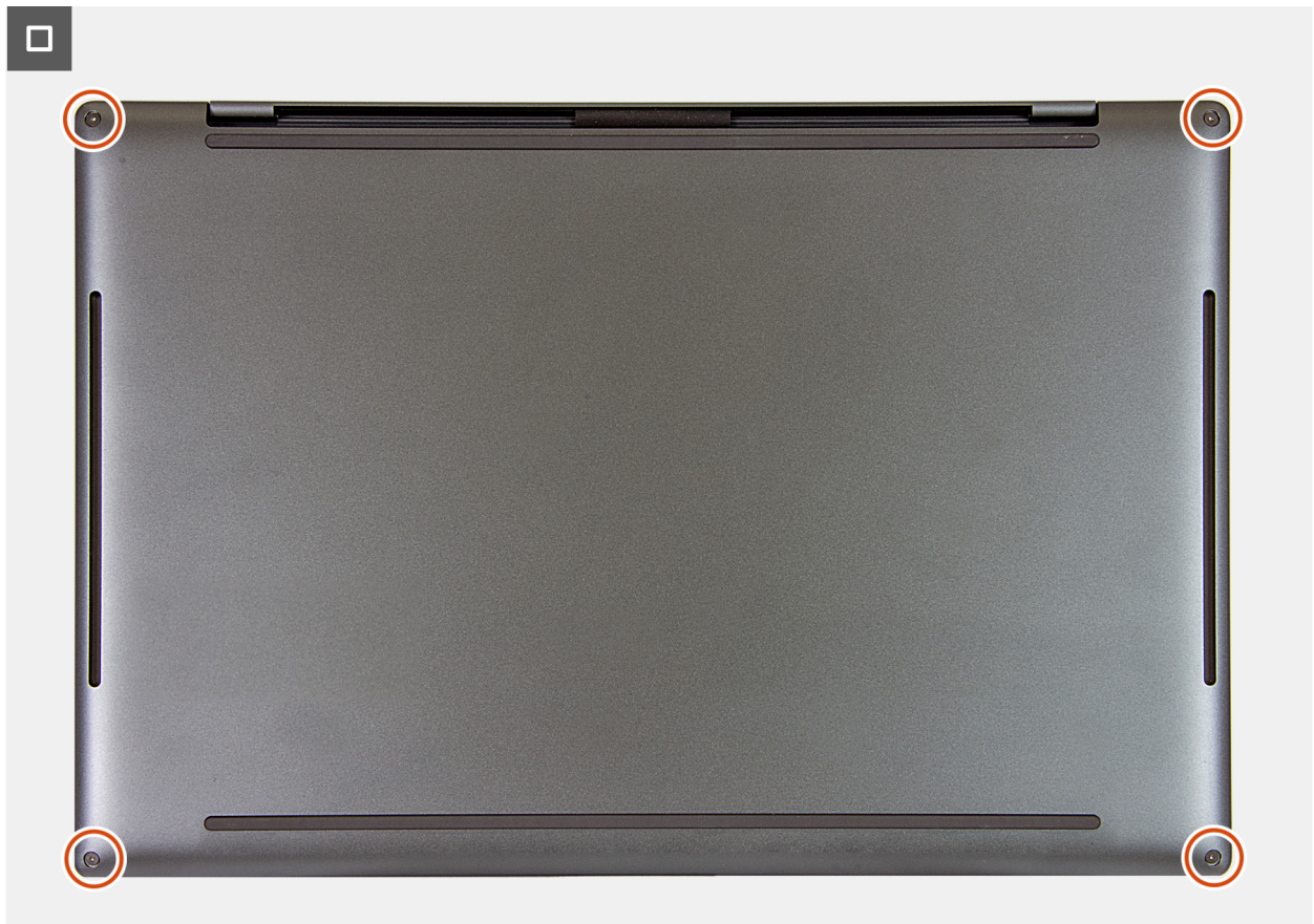
Figure 8. Tighten the four screws (M2x3.9, Torx 5) that secure the base cover to the palm-rest and keyboard assembly
