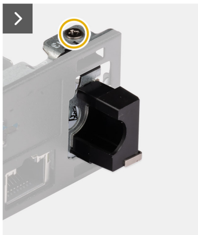
Figure 32. Installing the antenna module (white cable)
