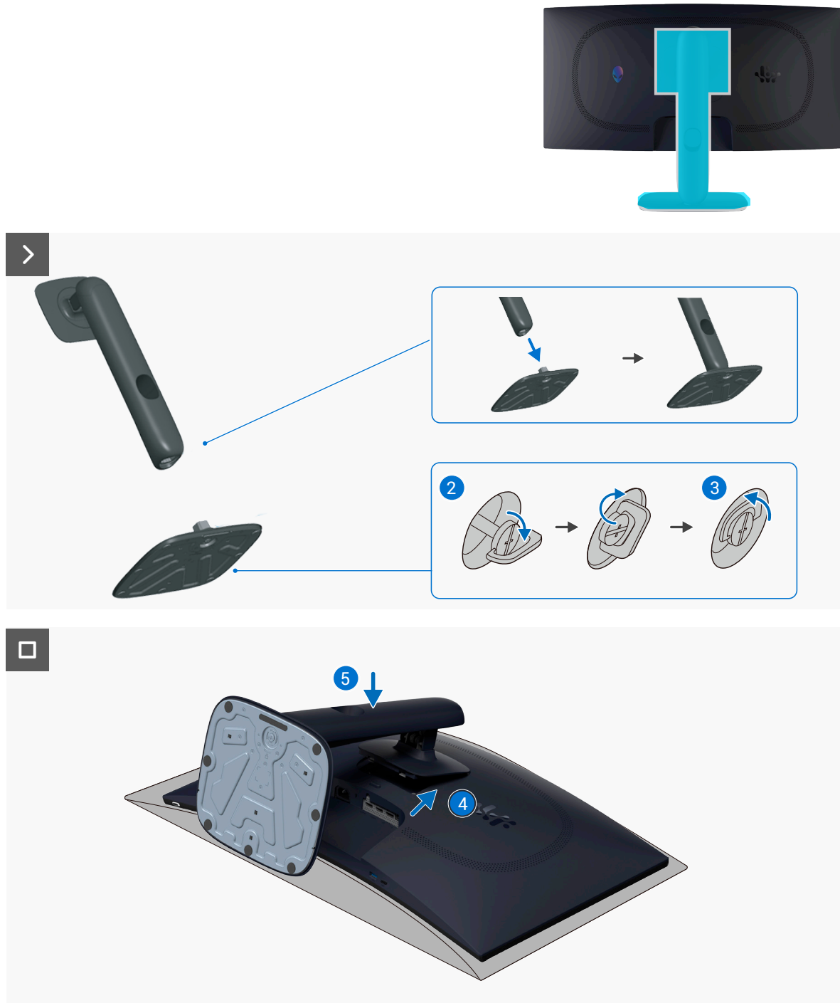
Figure 15. Installing the stand
