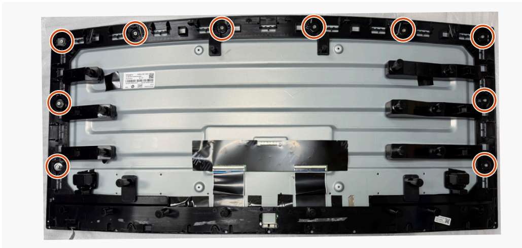
Figure 33. Removing the middle frame
