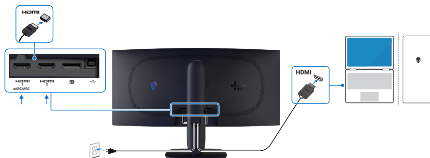
Figure 10. Connecting the HDMI cable
