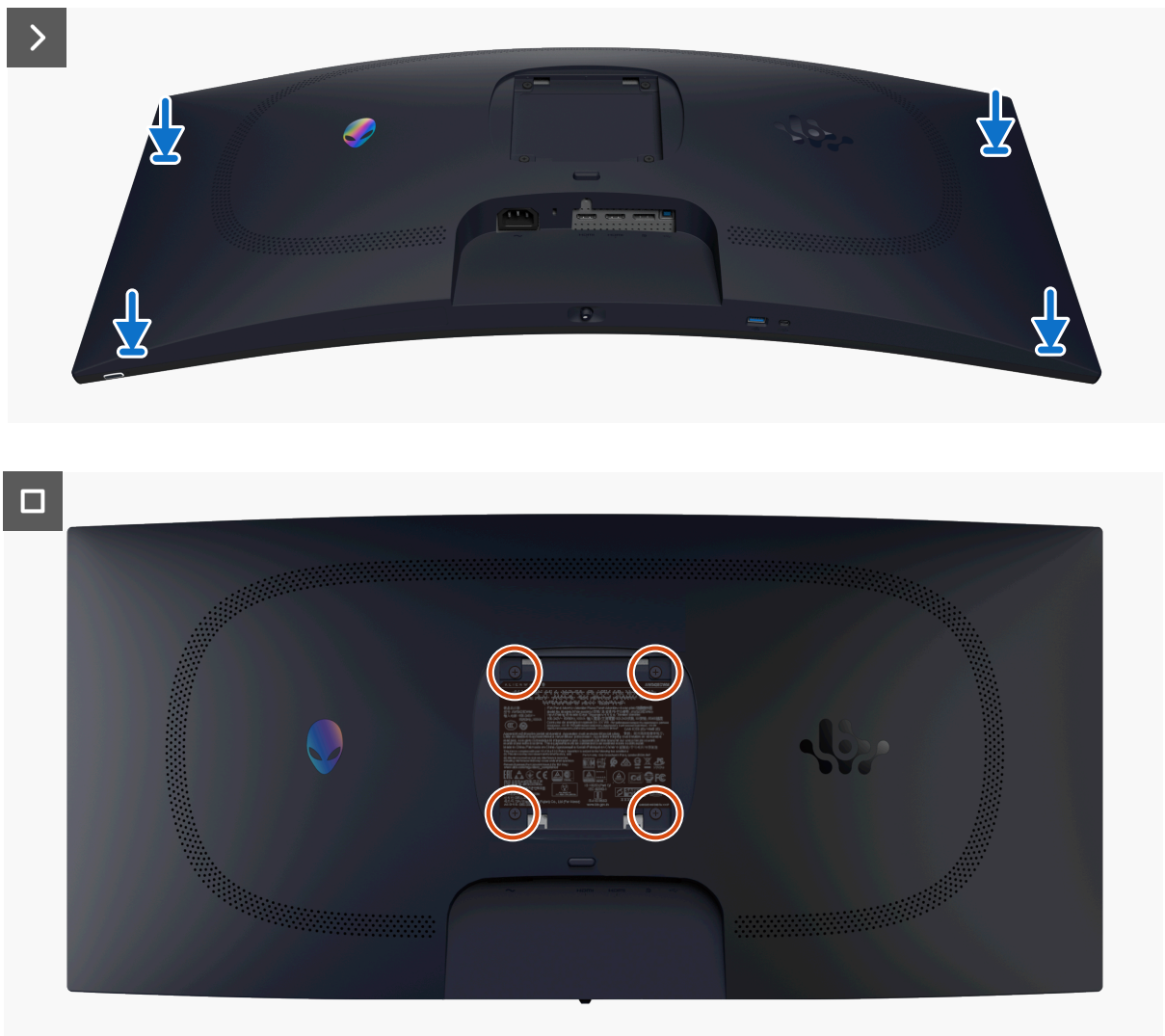
Figure 20. Installing the back cover
