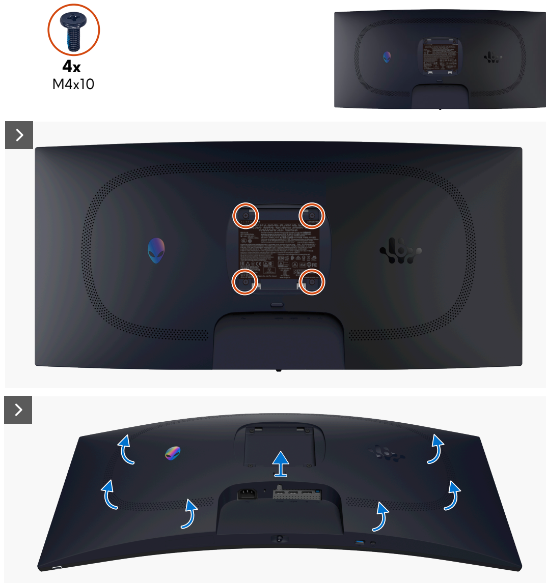
Figure 17. Removing the back cover
