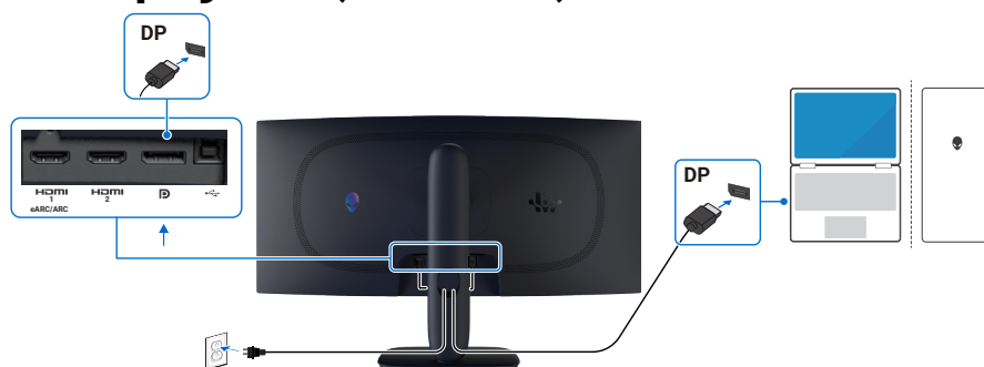
Figure 9. Connecting the DisplayPort (DP to DP) cable
