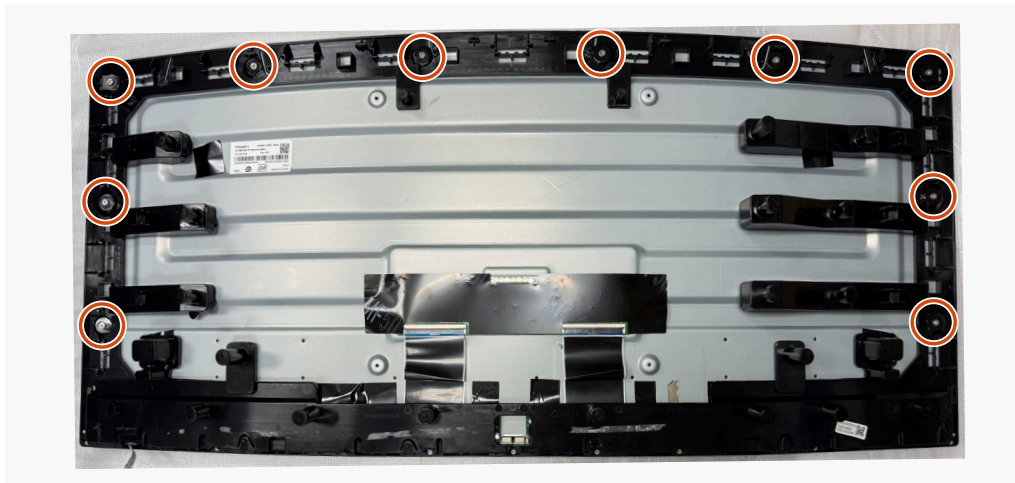
Figure 21. Installing the middle frame
