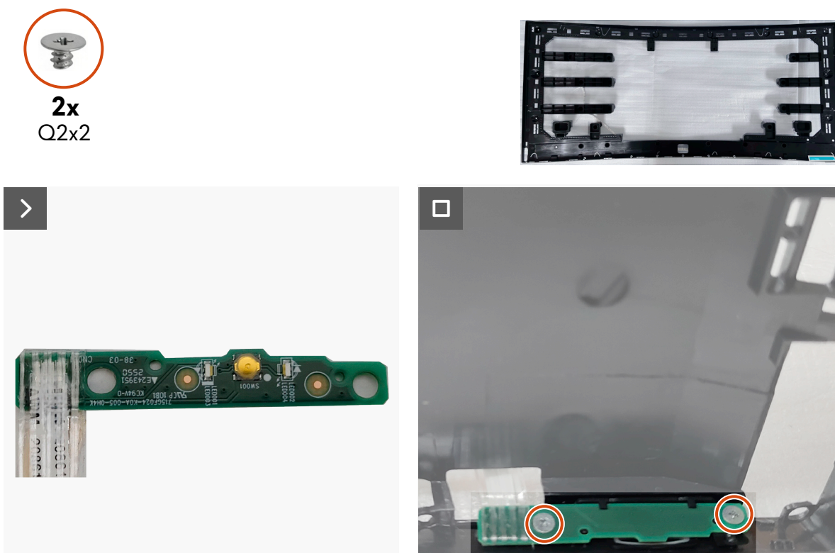
Figure 25. Installing the power-button board
