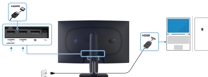
Figure 25. Connecting the HDMI cable
