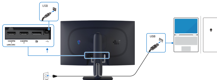
Figure 26. Connecting the USB Type-B (Type-B to Type-A) cable
