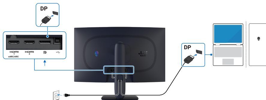
Figure 24. Connecting the DisplayPort (DP to DP) cable
