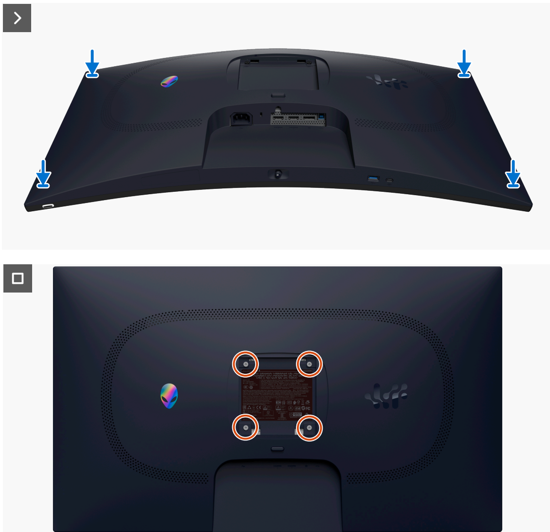
Figure 20. Installing the back cover
