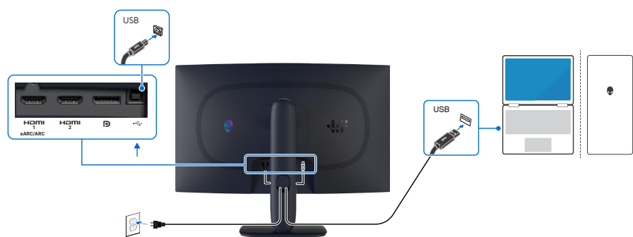
Figure 11. Connecting the USB Type-B (Type-B to Type-A) cable
