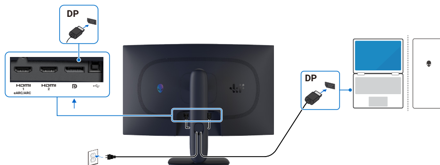
Figure 9. Connecting the DisplayPort (DP to DP) cable
