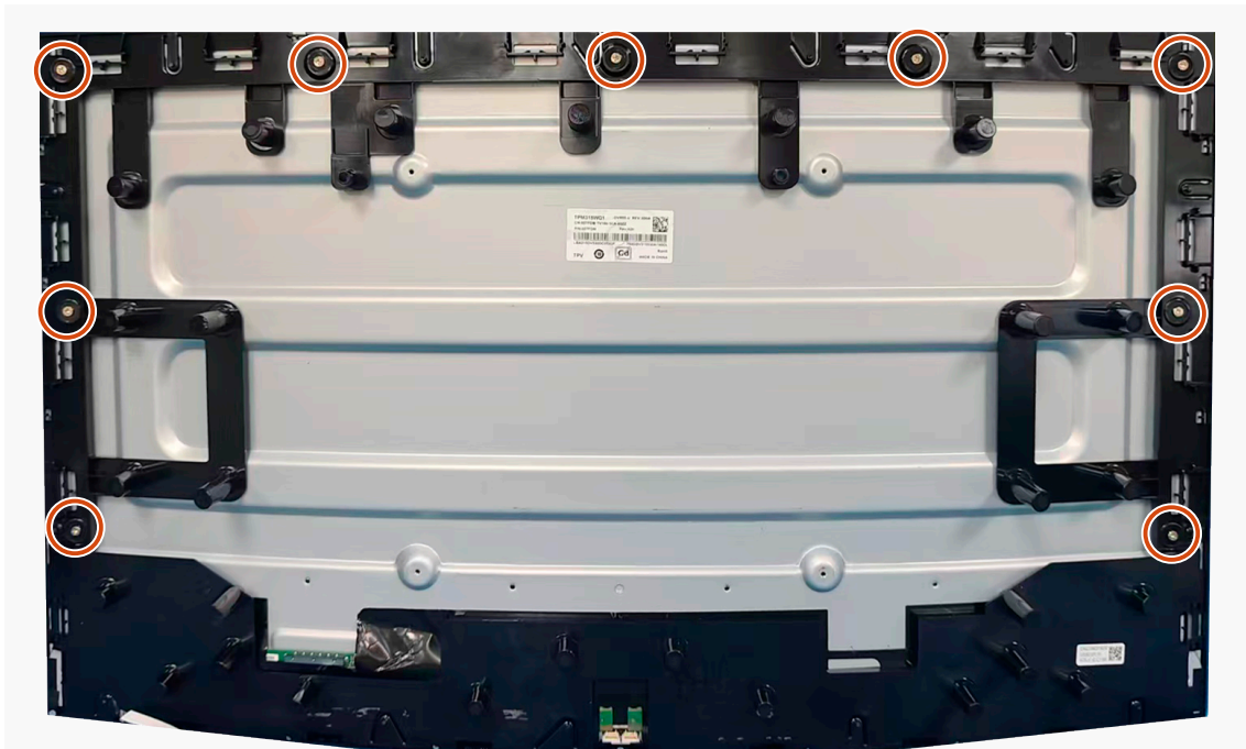
Figure 36. Installing the middle frame
