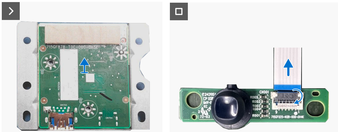
Figure 22. Removing the I/O board and joystick-button board
