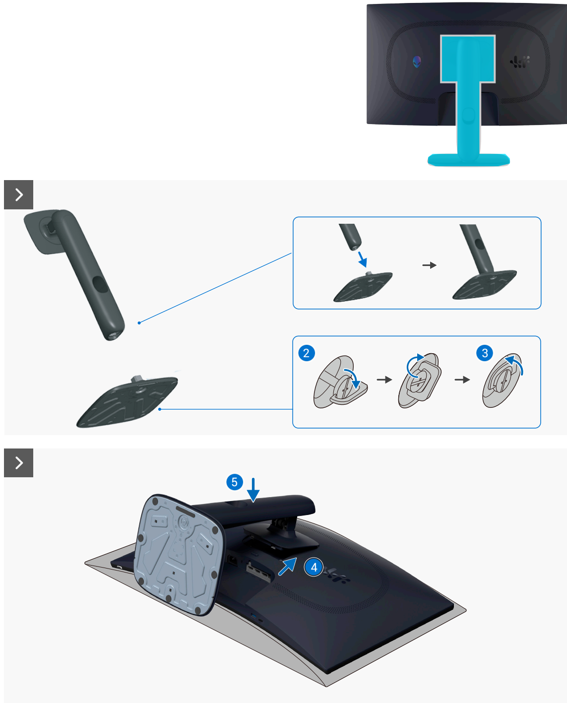
Figure 15. Installing the stand
