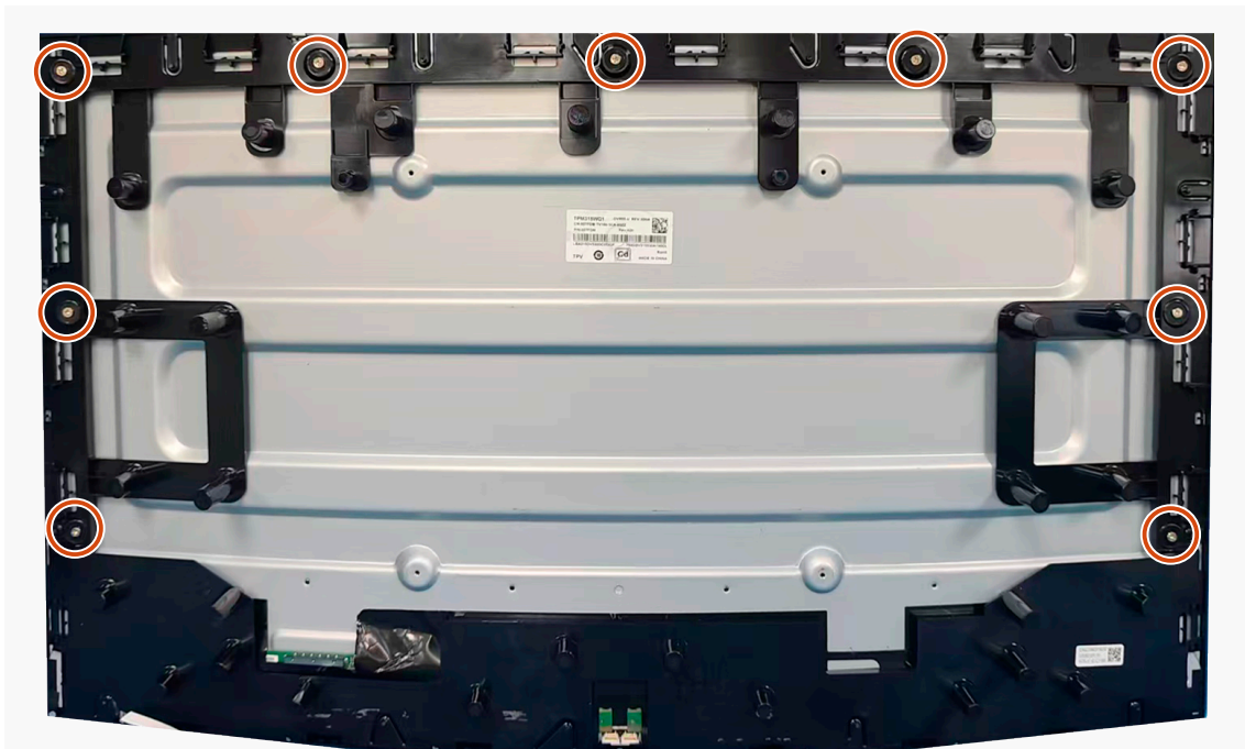
Figure 35. Removing the middle frame
