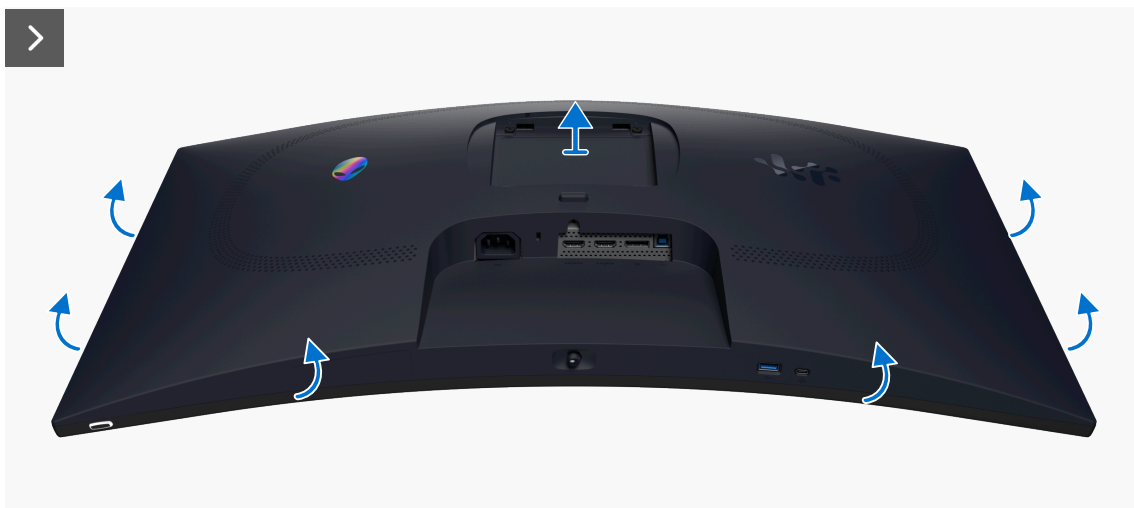
Figure 17. Removing the back cover
