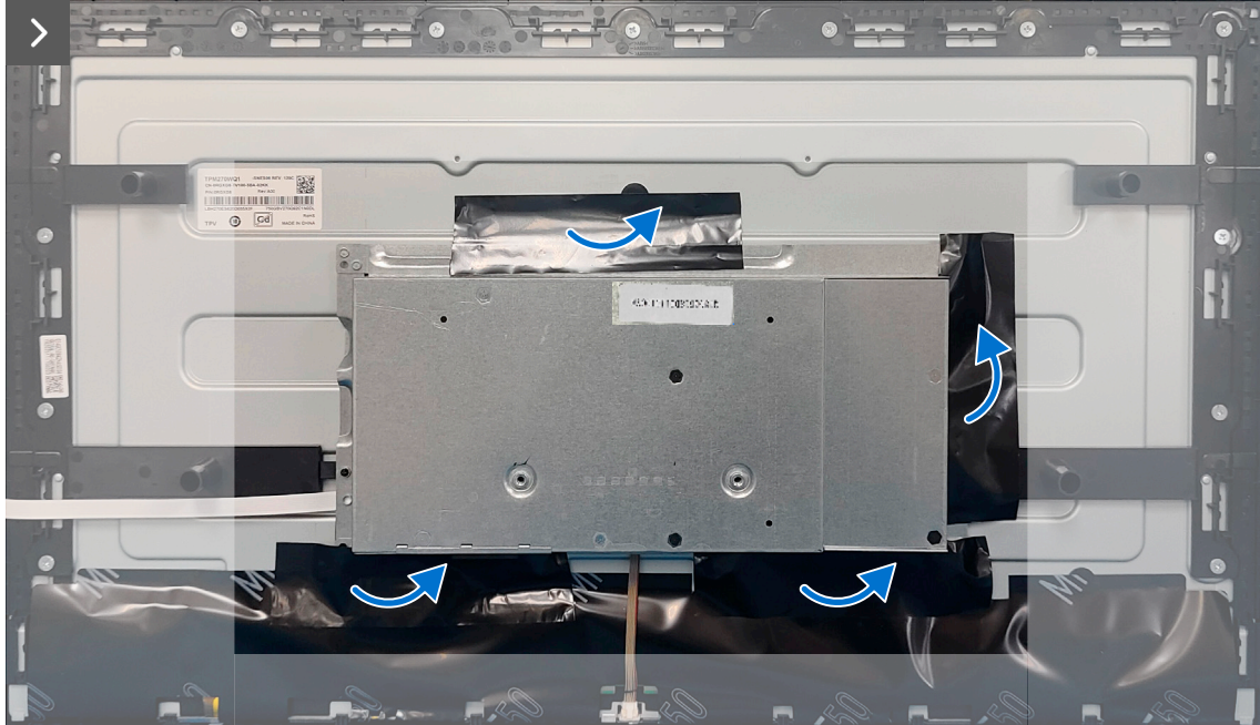
Figure 16. Removing the metal shield (AW2726DL)
