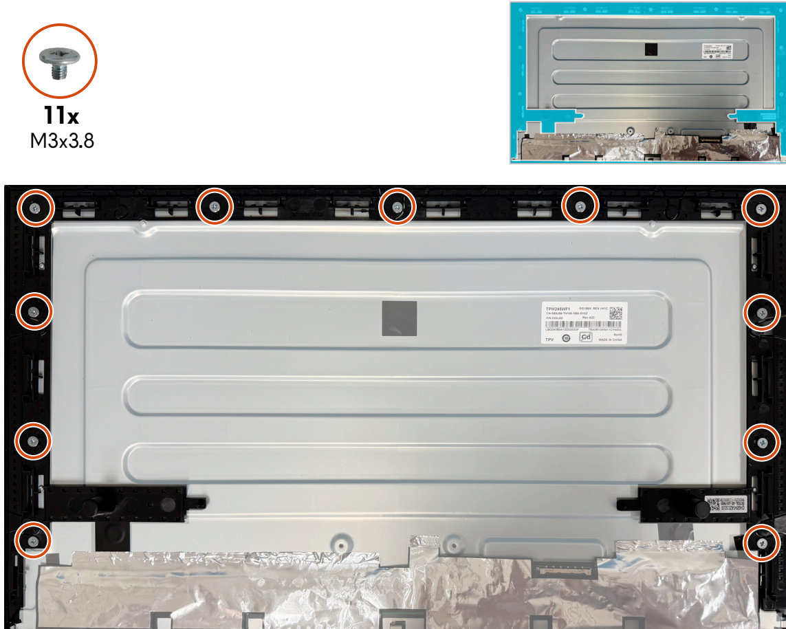
Figure 30. Removing the middle frame (AW2526HL)
