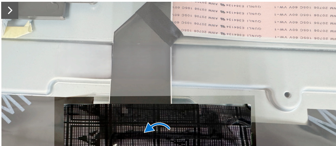
Figure 20. Installing the metal shield (AW2726DL)
