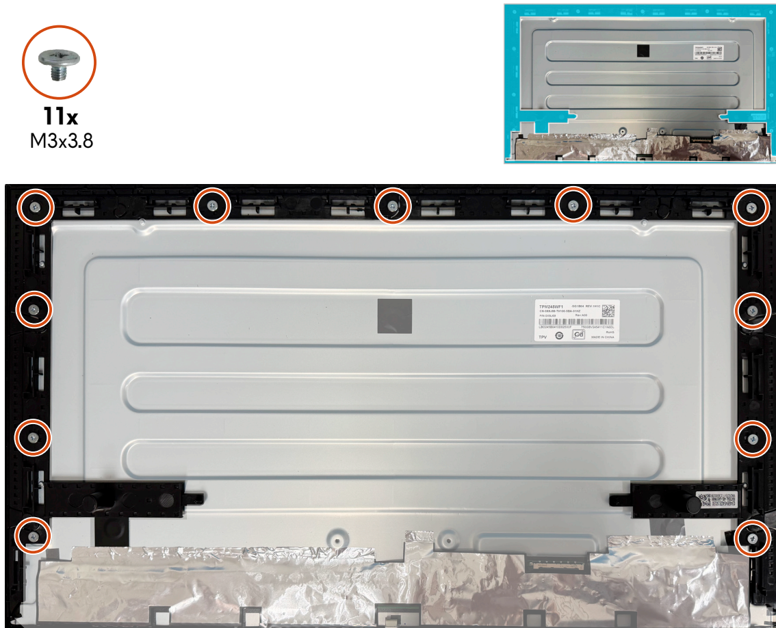
Figure 46. Installing the middle frame (AW2526HL)
