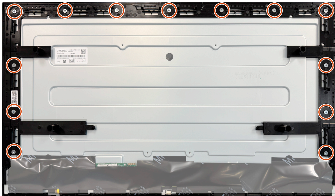
Figure 47. Installing the middle frame (AW2726DL)
