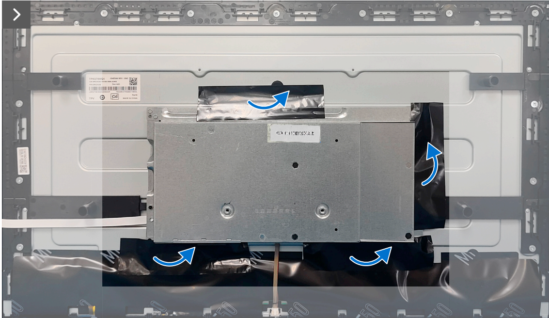
Figure 30. Removing the metal shield (AW2726DL)
