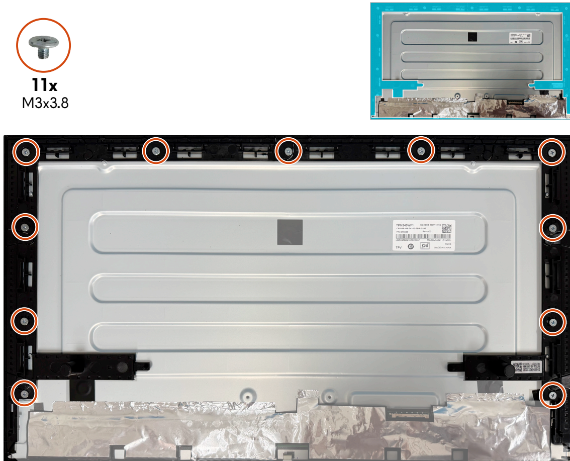
Figure 44. Removing the middle frame (AW2526HL)
