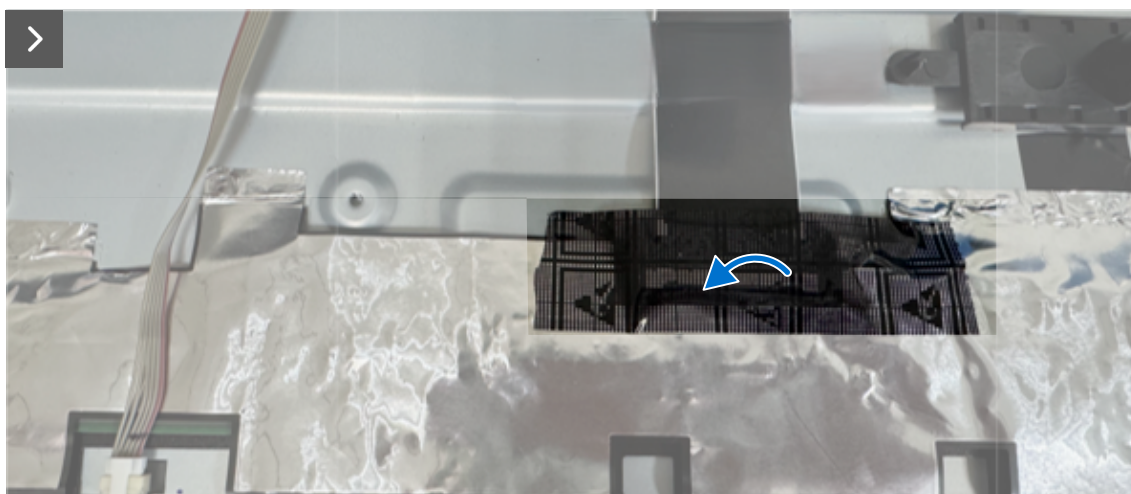
Figure 32. Installing the metal shield (AW2526HL)
