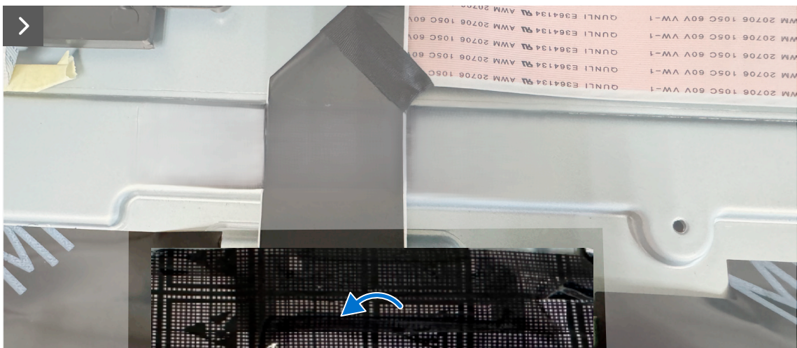
Figure 34. Installing the metal shield (AW2726DL)
