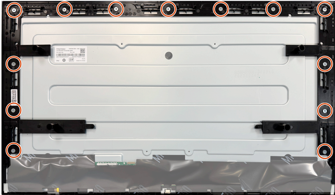
Figure 45. Removing the middle frame (AW2726DL)
