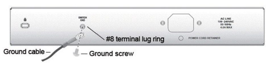
Figure 2.10 – Connect a Grounding Cable
