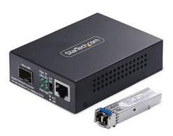
This Gigabit Ethernet to fiber media converter offers a reliable way to extend your network up to 20 km (12.4 mi) using single-mode LC fiber, providing increased range, enhanced security, and reduced interference compared to copper-based connections. It's TAA compliant and designed for government and commercial applications where long-distance and rack-mountable fiber access is needed.
