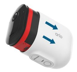
2. Align the battery and insert it into the battery compartment.
