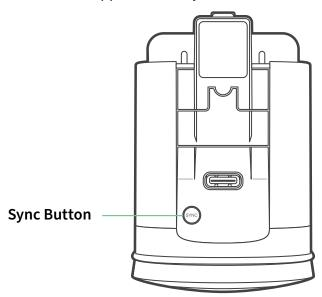
The Arlo Secure App should detect your camera automatically. Once it does, follow the instructions in the Arlo Secure App to pair and install the camera. When the camera is shut down, pressing the Sync button does the following:
