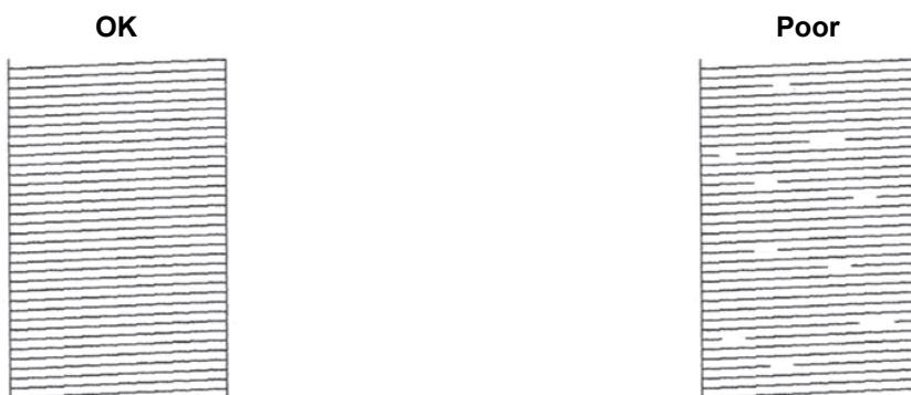
5. When the LCD message prompts you to check the print quality of each colour, press the number of the pattern (1–4) that most closely matches the printing result.
