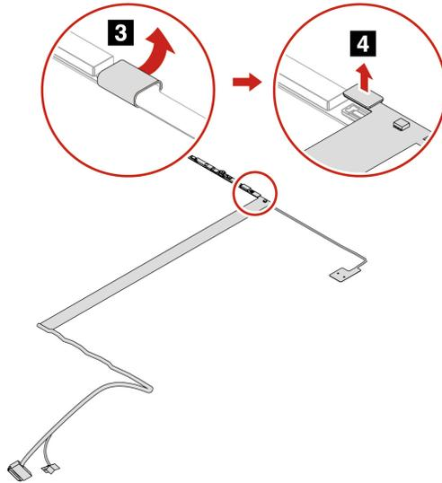
Step 3. Install the camera-and-microphone-module in reverse order.
