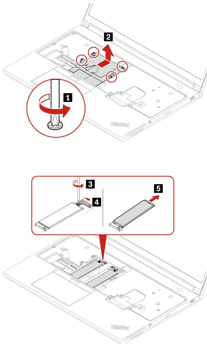
2. Install the M.2 solid-state drive and M.2 solid-state drive bracket in reverse order.
