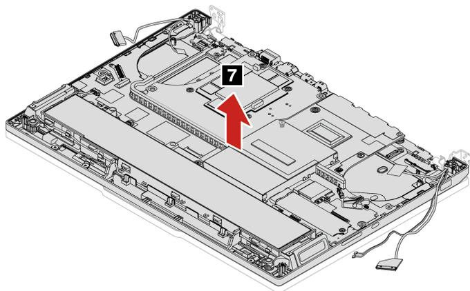
Step 2. Install the LCD unit in reverse order. When installing, ensure that the connectors are attached firmly.
