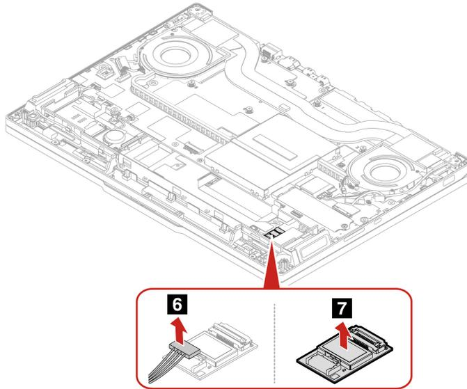
Step 2. Install the NFC cable and NFC board in reverse order.
