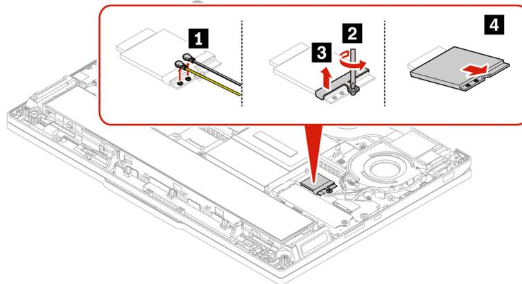
Step 2. Install the wireless LAN module in reverse order.
