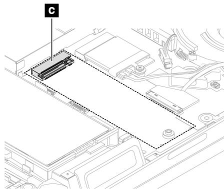
**M.2 solid-state drive and M.2 solid-state drive bracket under the keyboard**
