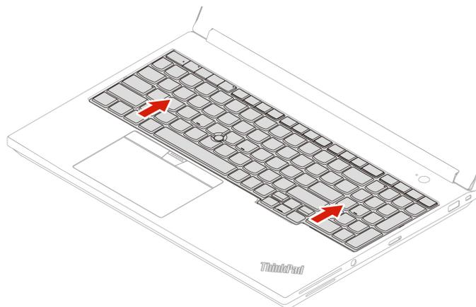
Step 3. Pivot the keyboard slightly upward **1** and then turn the keyboard over **2**.
