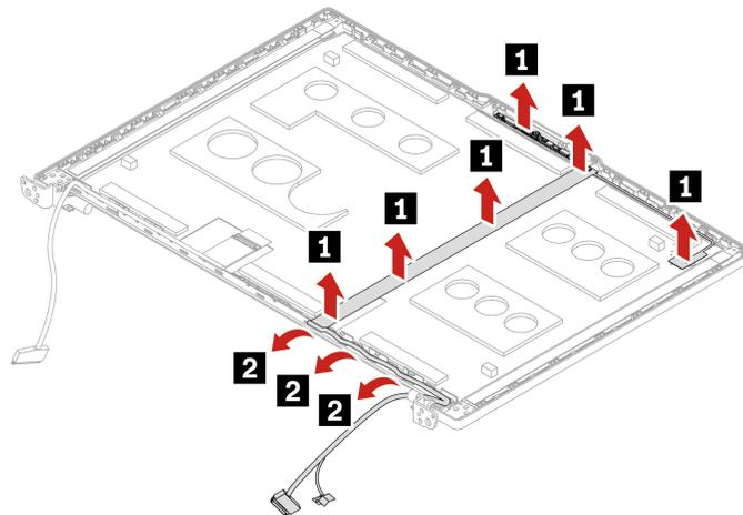
Step 2. Remove the camera-and-microphone-module cable as shown below.
