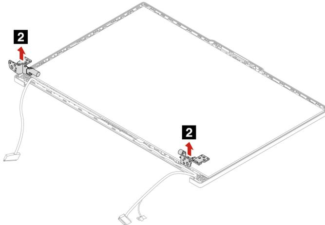
Step 2. Install the LCD hinges in reverse order.
