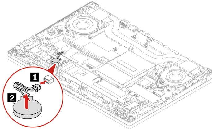
Step 2. Install the coin-cell battery in reverse order.
