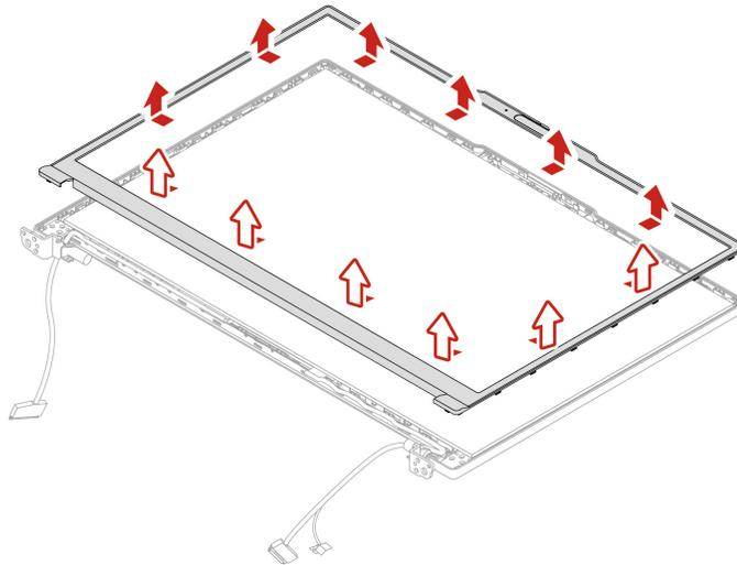
Step 2. Install the LCD bezel in reverse order. When installing, ensure that all the latches are attached firmly.
