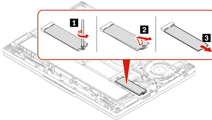
2. Install the M.2 solid-state-drive and M.2 solid-state drive bracket as shown below.
