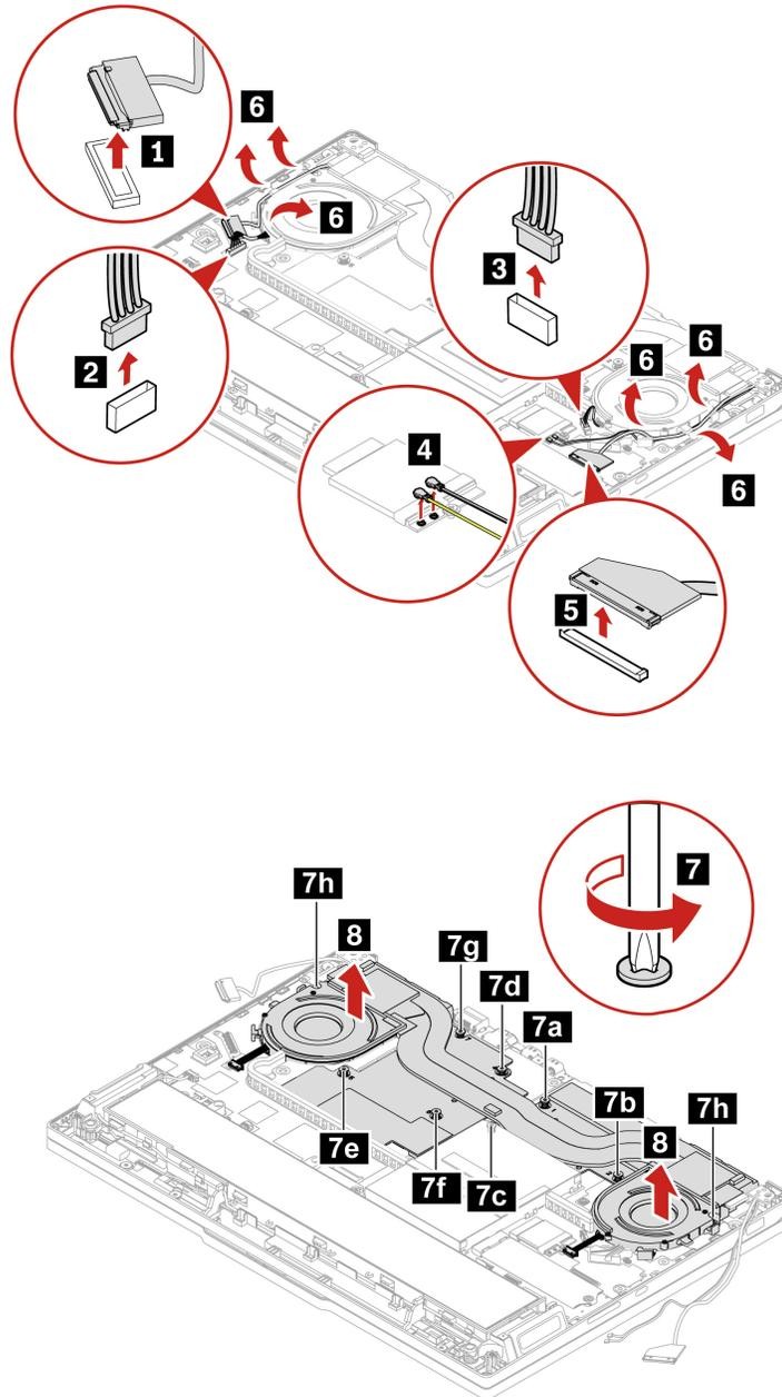
Step 2. Install the thermal fan assembly in reverse order.
