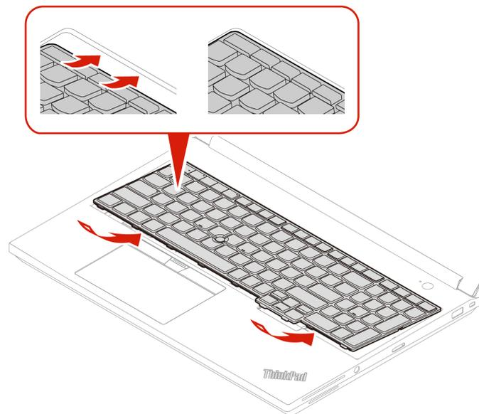
Step 3. Slide the keyboard in the direction as shown. Ensure that the latches are secured under the keyboard frame.
