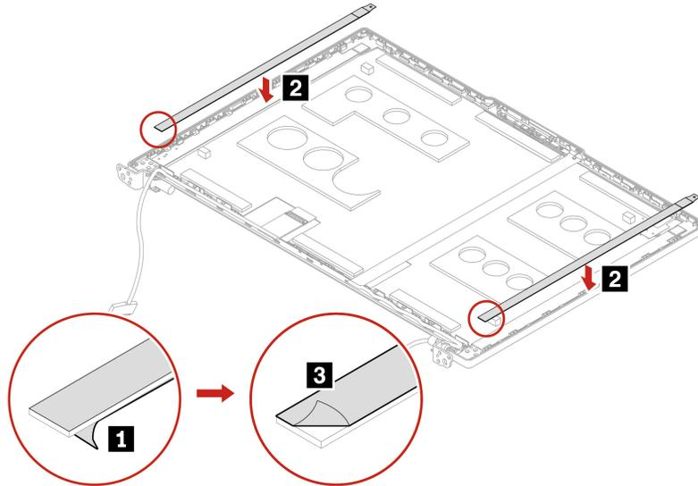
Step 2. Attach the LCD cable to the LCD panel as shown. Turn over the LCD panel to secure the LCD panel with tapes.
