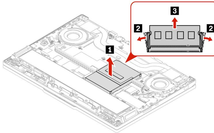
Step 2. Install the memory module as shown below.
