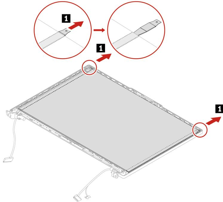
Step 2. Turn over the LCD panel and detach the LCD cable from the LCD panel as shown.
