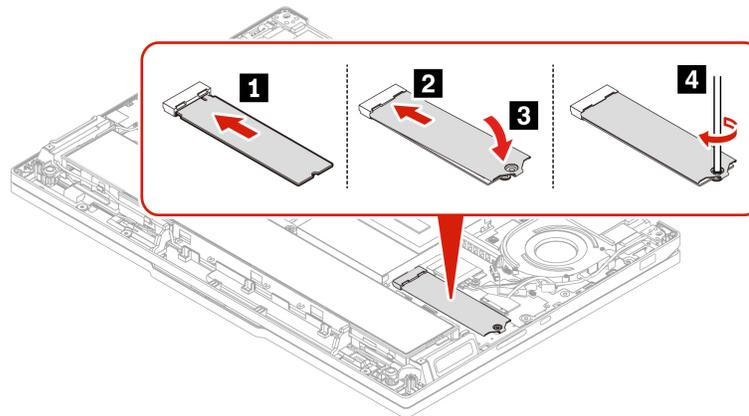
**Note:** During the M.2 solid-state drive replacement, if the thermal pads require reapplication or replacement, ensure the adhesive side is attached to the system board or M.2 solid-state drive brackets.
