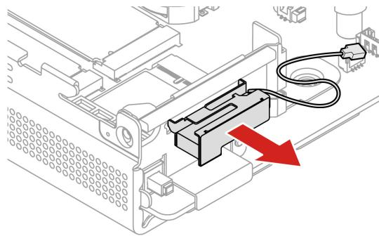
2. Align the two feet of the front Wi-Fi antenna with the two holes on the antenna bracket and install the front Wi-Fi antenna to the antenna bracket.
