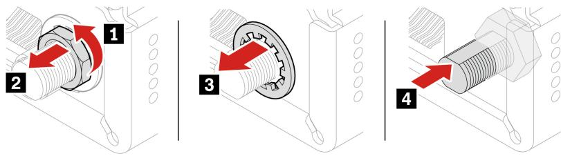
2. Install a new rear Wi-Fi antenna in reverse order.
