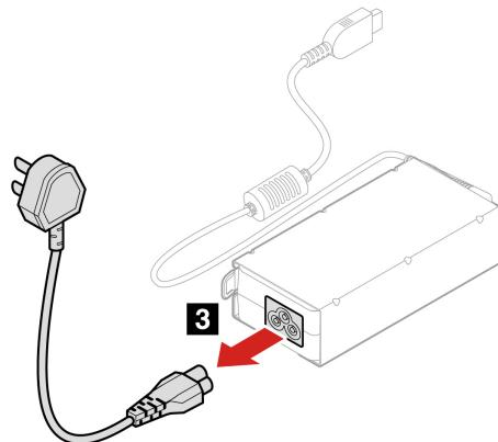
3. Push the ac power adapter out of the power adapter bracket. Remove the ac power adapter.
