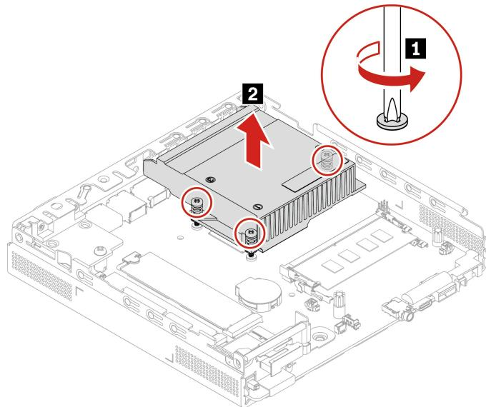
3. Install a new CPU heat sink in reverse order.
