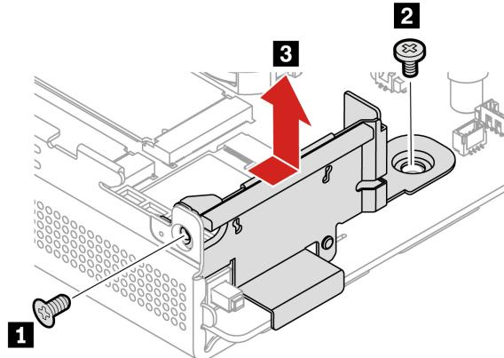
3. Install a new antenna bracket in reverse order.
