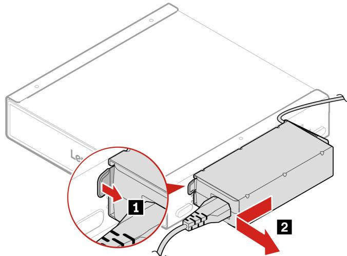
2. Disconnect the power cord from the ac power adapter.
