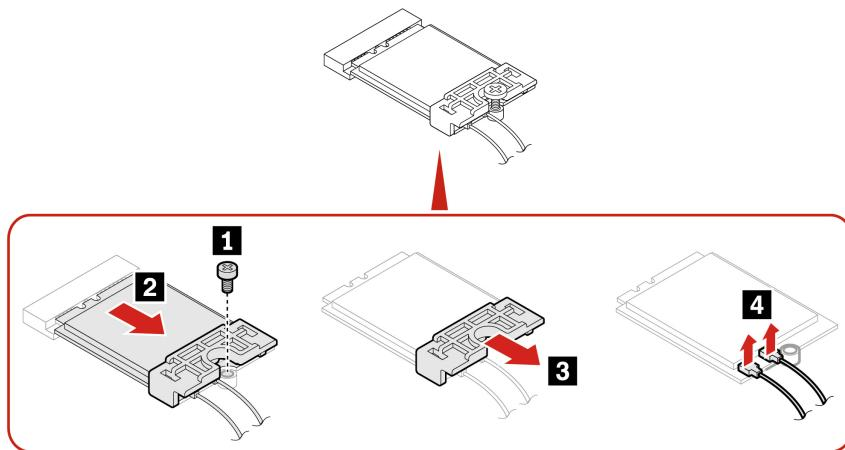
3. Install a new Wi-Fi card or Wi-Fi card shield in reverse order.
