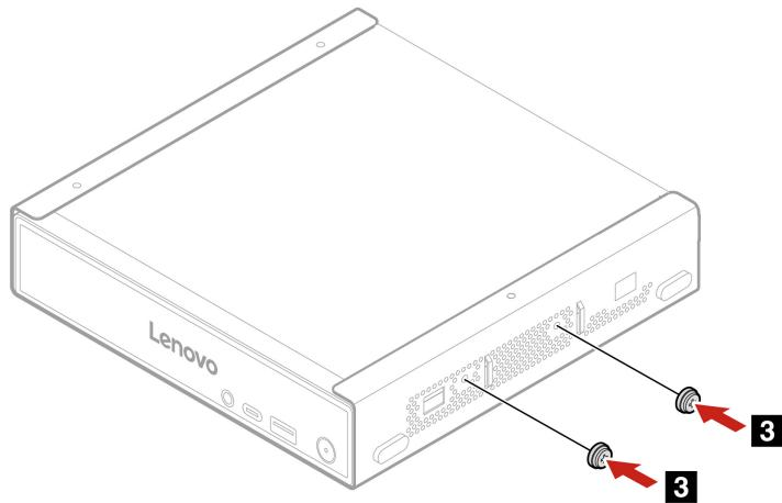
4. Align the two holes on the power adapter bracket side to the two screws on the VESA mount bracket side. Pull the power adapter bracket backward to secure it on the VESA mount bracket.
