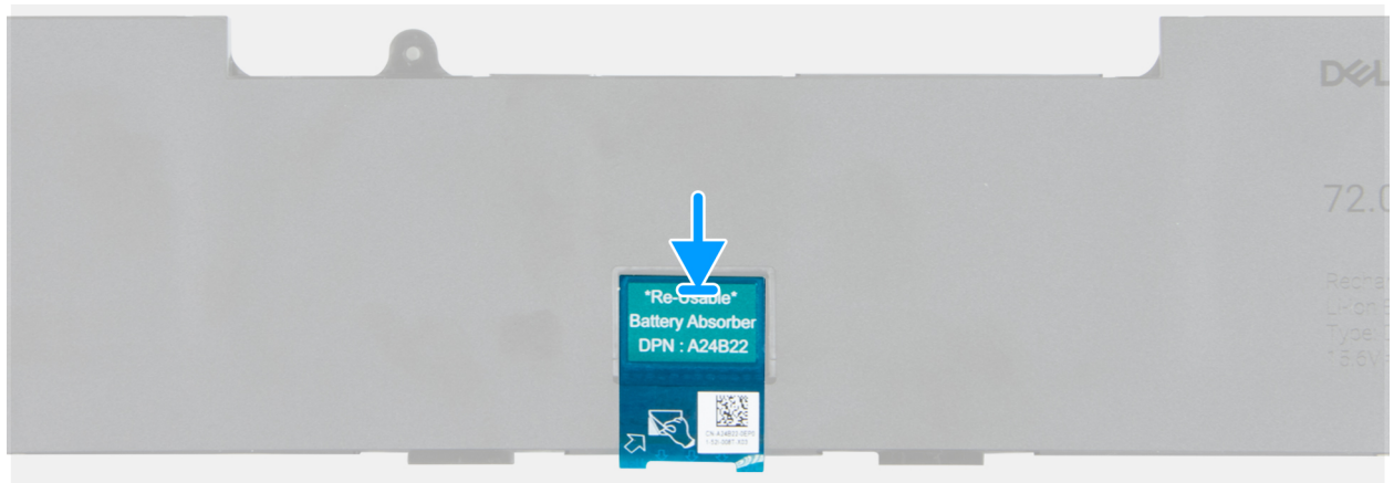
Figure 20. Installing the battery absorber
