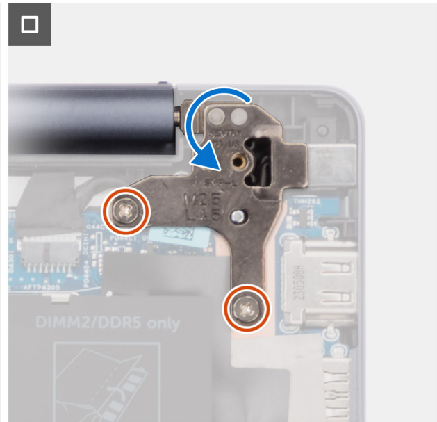
Figure 40. Installing the power-adapter port (for computers shipped with an aluminum chassis)
