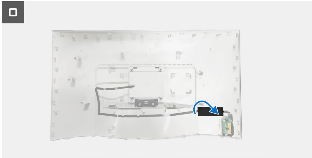
Figure 13. Installing the keypad board
