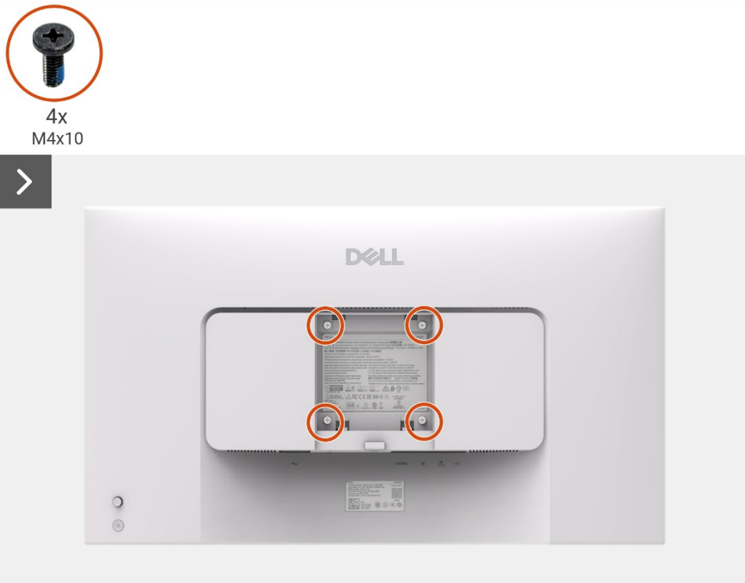
Figure 16. Removing the back cover
