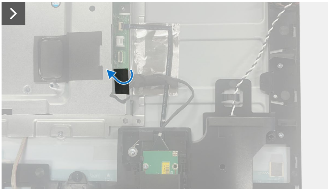
Figure 28. Removing the QAP board
