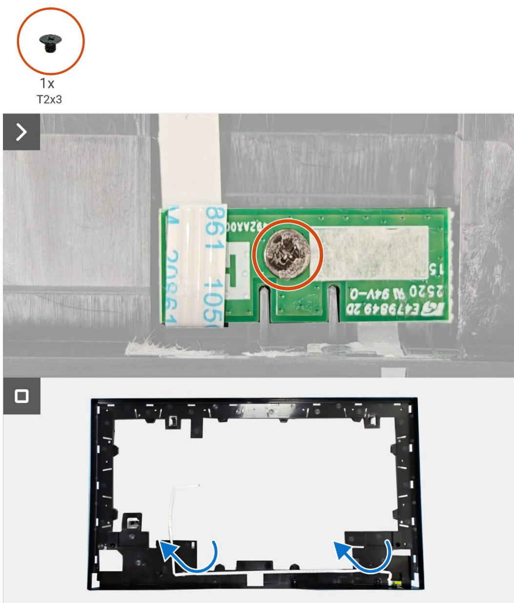
Figure 49. Removing the LED board
