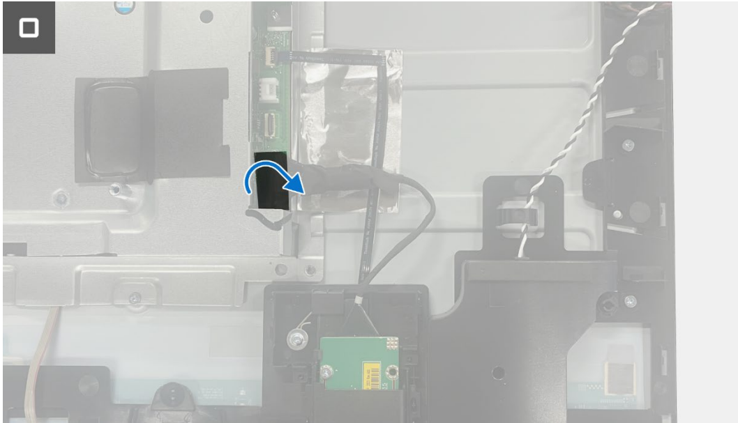
Figure 33. Installing the QAP board
