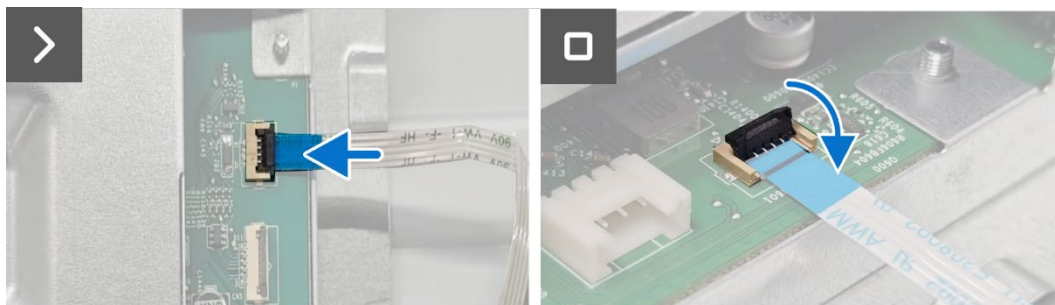
Figure 39. Installing the chassis assembly
