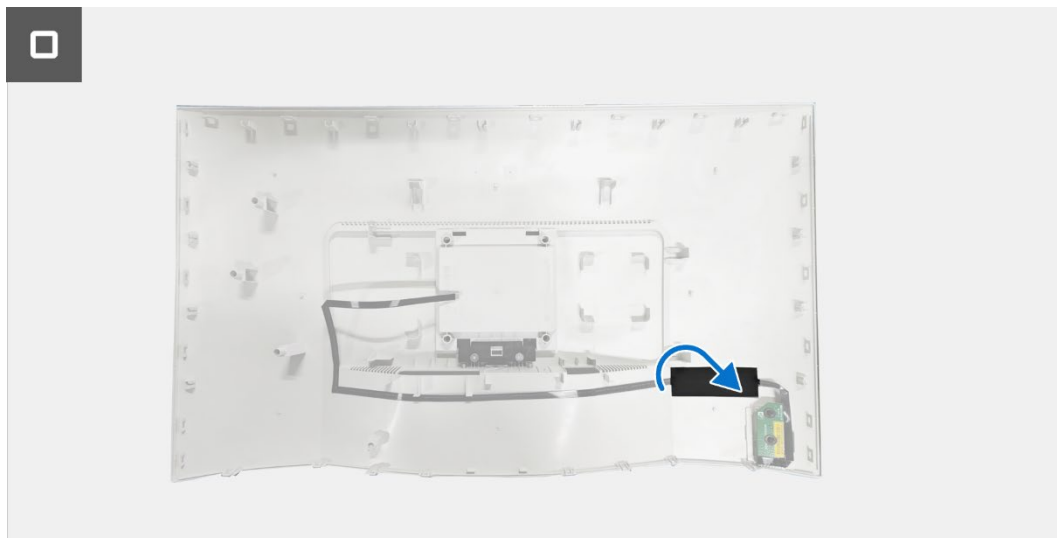
Figure 23. Installing the keypad board
