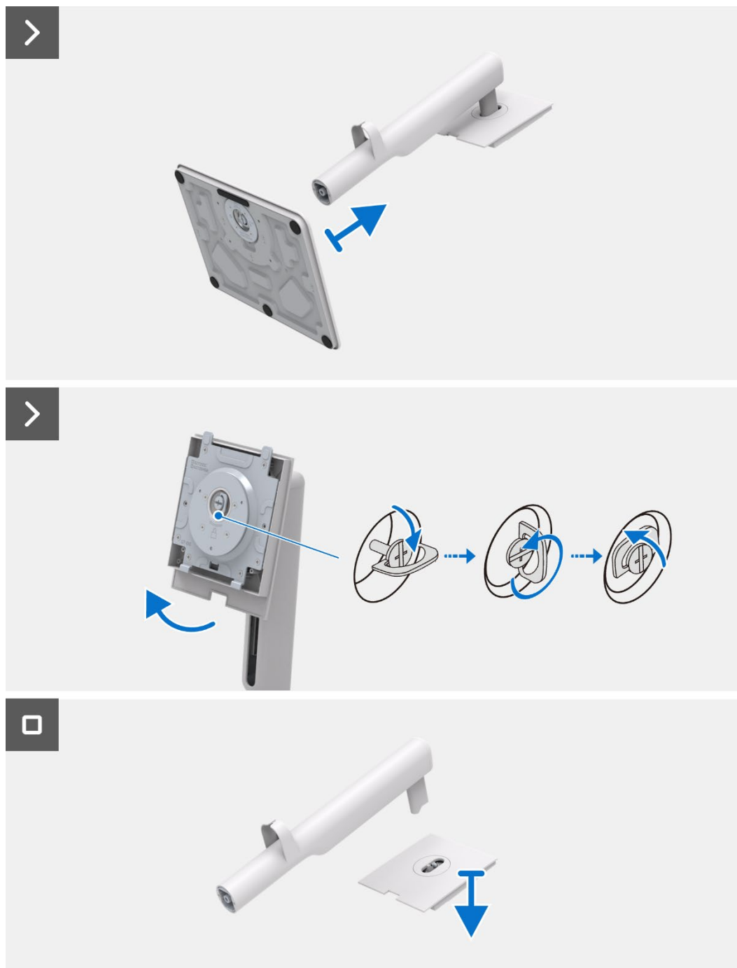
Figure 12. Removing the stand
