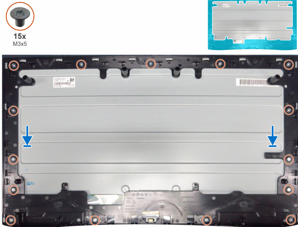
Figure 13. Installing the middle frame for S2425HSM
