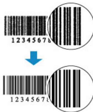
Printed Barcodes Are Not Recognized
