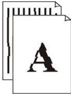
Lines Are Misaligned/Distorted
