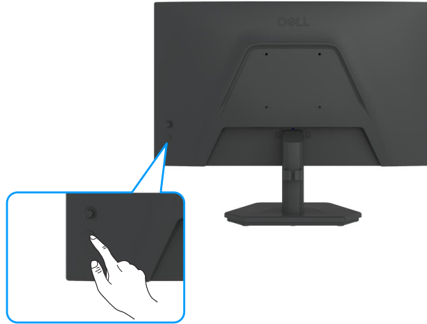
Figure 19. Power on the monitor
