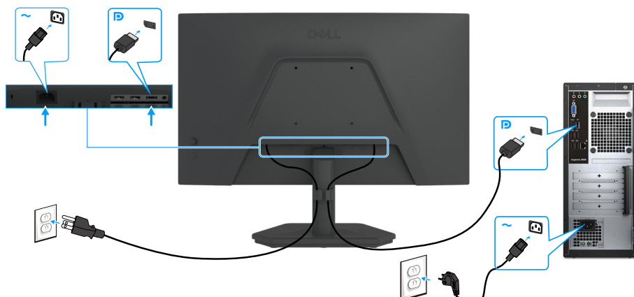
Figure 15. Connecting the DisplayPort cable
