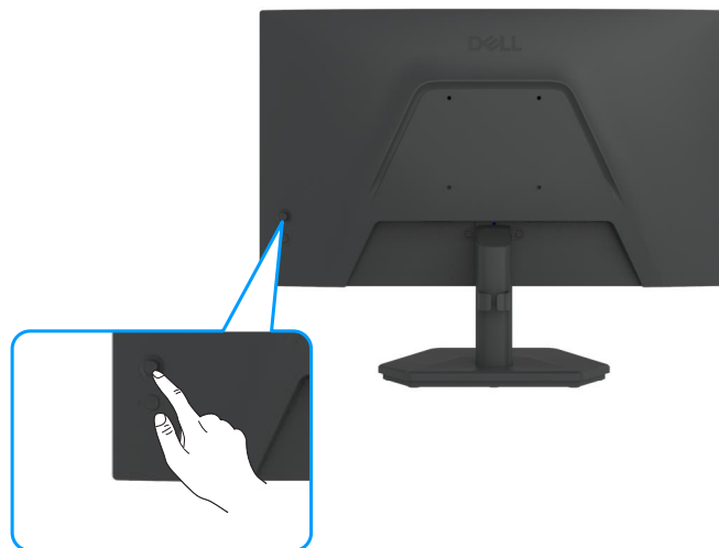
Figure 20. Using the joystick control
