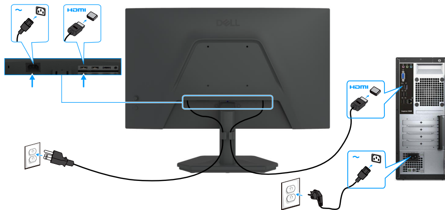
Figure 14. Connecting the HDMI cable
